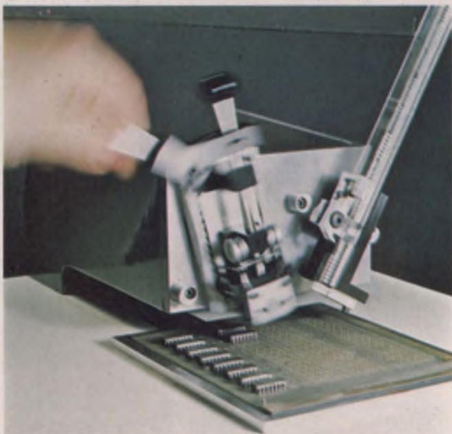
Don't let the chips fall where they may! Dual, in-line integrated-circuit packages permit the user to design equipment assemblies. The semi-automatic inserting tool quickly and easily places IC packages directly on printed-circuit boards, lowering manufacturing cost and time.
