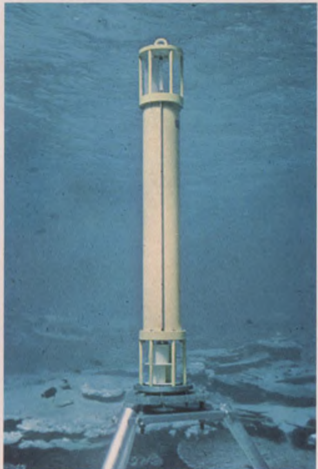
Instrument package developed by Bissett-Berman Corp. for measuring salinity and temperature at various depths.
