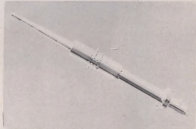
5. Radial mounting of diodes in a microwave switch or limiter increases the device's power-handling capability. This coaxial switch covers the frequency range of from 1 to 4.5 GHz and can switch 30 kW peak and 30 watts average power in 200 ns.
