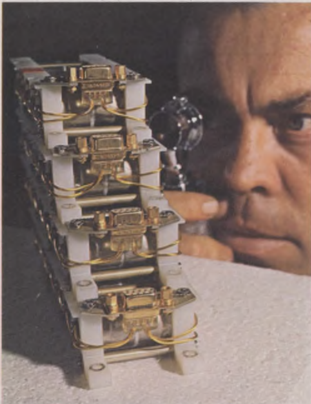
Gold-plated wiring harness connectors shown mounted on nickel-cadmium batteries carried in the Syncom communications satellite. Similar installation was used in the Early Bird satellite, and advanced version of Syncom.
