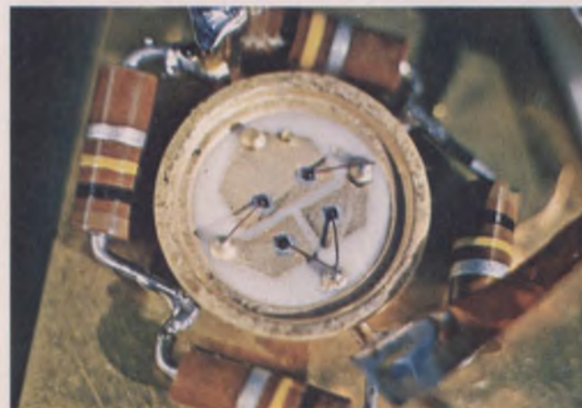
Varactor quad under development. Its optimum dc return resistance has to be determined experimentally so that it can be integrated with varactors.
