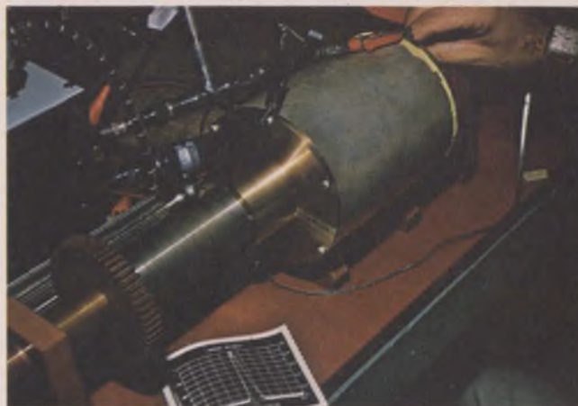
High-Q cavity reduces noise of cw Gunn oscillators. However, the cavity is large and not tunable electronically.
