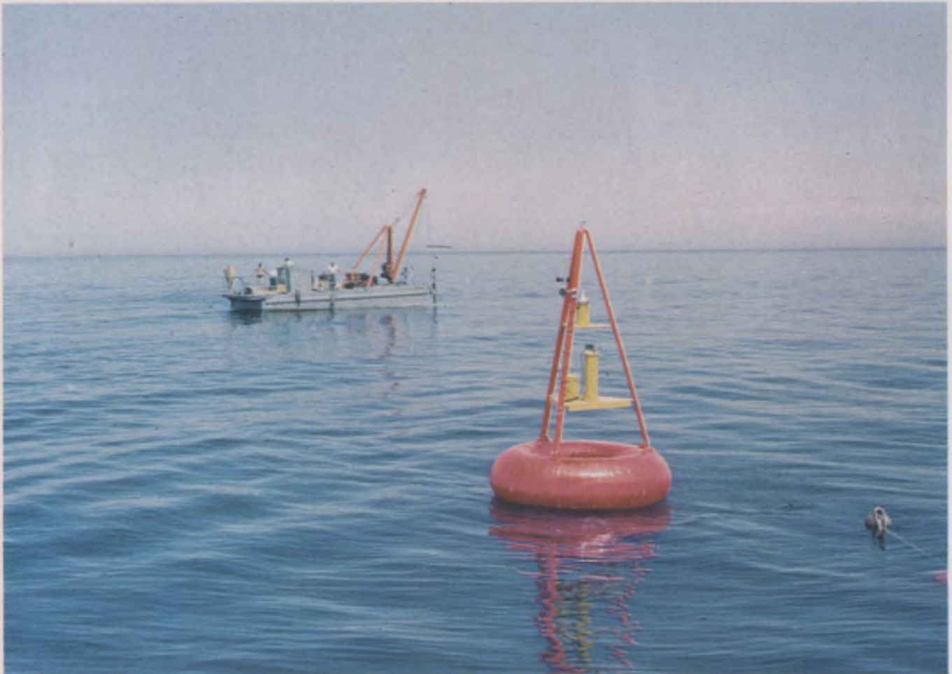
Flotation buoy built by Geodyne Corp. supports three current meters and three temperature recorders below the
