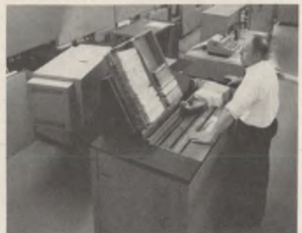
Electro-optical reader tackles zip-codes in Detroit post office. Scanning head (under worker's right hand) reads as fast as 15 men.
