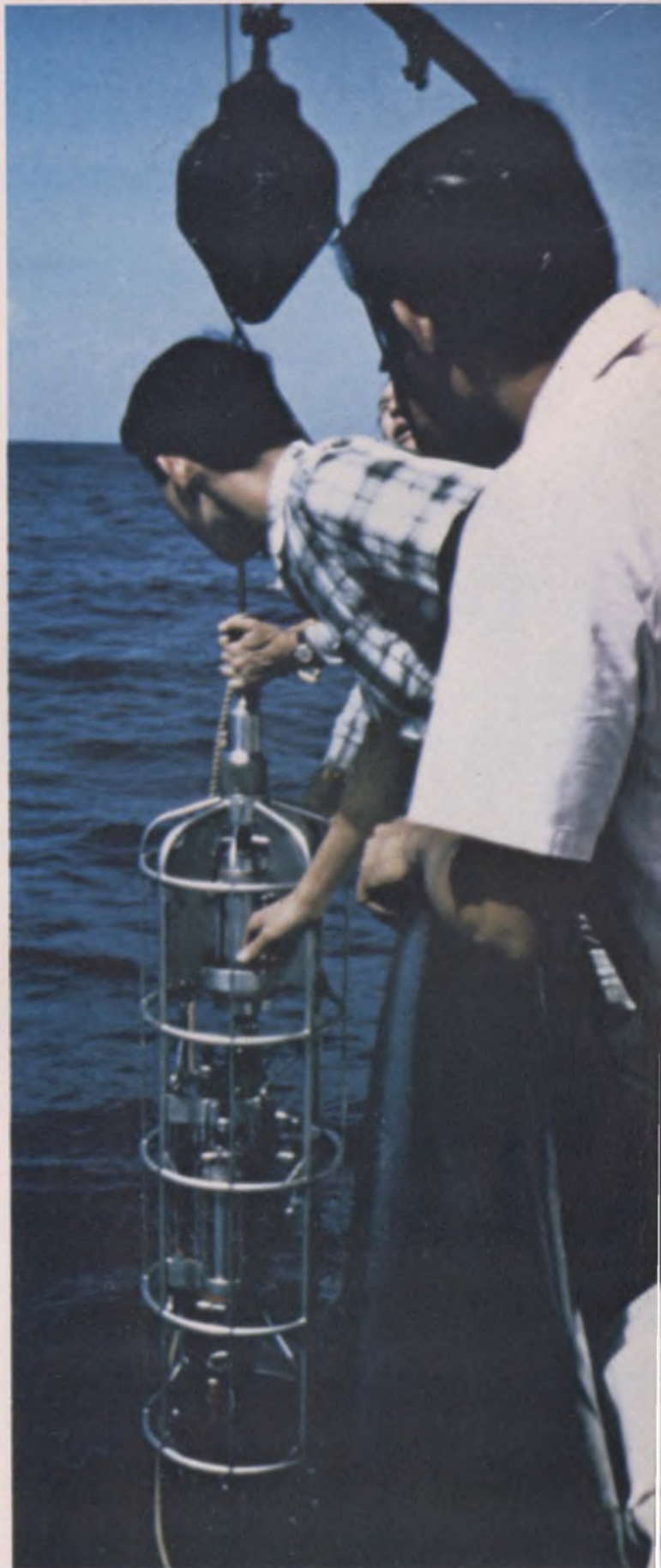
Underwater instrument measures tidal currents near the ocean's floor. Electronics are used for recording the data and telemetering it back to the surface.
