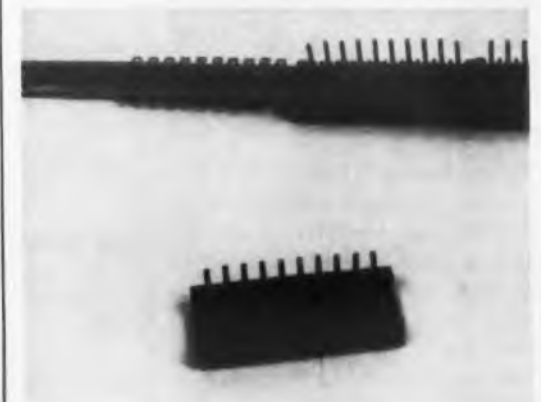
Fig. 1. Sandwich bus has bonded layers of copper strip and 5-mil insulation.
