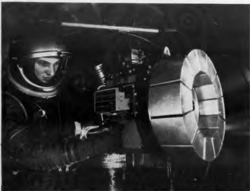
Pinched plasma electromagnetic engine for such space missions as satellite spin-rate stabilization and orbit modification generates thrust by ejecting a plasma beam, accelerated by the interaction of a self-induced magnetic field and electrical skin currents. Capacitor at left is charged by a novel converter capable of constant-current charging. Pressure bottle holds two-year supply of nitrogen fuel.
