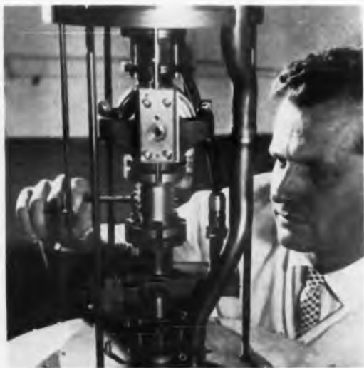
Extended-interaction circuit to increase power, efficiency and bandwidth of klystrons is tested in laboratory of Sperry Gyroscope Co. Circuit makes use of rods inserted transversely in klystron waveguide to create standing-wave resonance on slow-wave line, eliminating resonant cavity.
