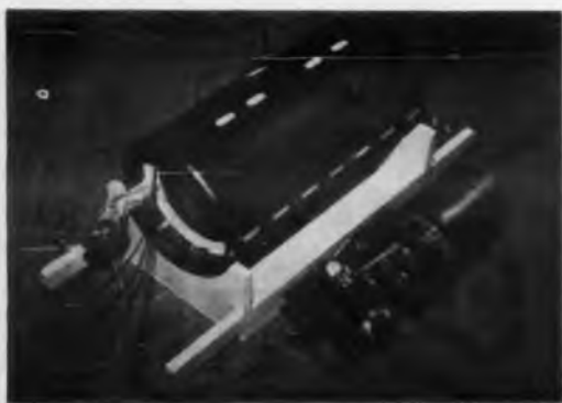
Titanium canister, left, houses telemetry recorder unit. White lining, at open end of canister, is insulating material. White ovals are transducers. At right, is fm/fm telemetry system and closed-loop magnetic tape recorder/reproducer.
