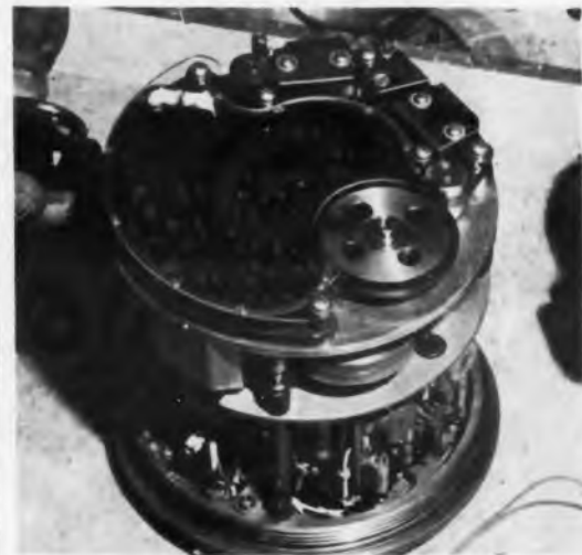
Magnetic tape in a continuous 25-ft loop is used in 6-lb recorder-reproducer. Tape speed is 5-1/2 in. per sec. It will record heat data when SNAP telemetry canister passes through transmission blackout area on return to earth.
