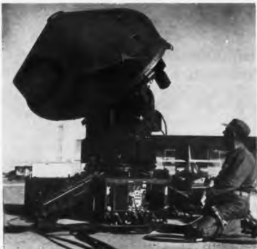
AN/TPQ-10 radar , to be used in automatic landing system for spacecraft and re-usable stages of missiles, can track a vehicle from 500 miles in space.
