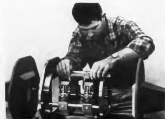
Perforated-plate Fabry-Perot interferometer for the 3- to 4-mm range is adjusted for parallelism by G. L. Strine. The device is being used as the cavity resonator in a hydrogen-cyanide gaseous maser.
