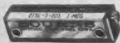
General-Purpose Resiston® Carbon Trimpot®—Model 215. Operates to 125°C / L, S, P terminals / ¼ watt / 20K to 1 Meg. Unsealed.
