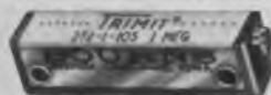
High-Quality, Low Cost Commercial Carbon Trimpot®—Models 272, 274, 276. Operates to 85°C / L, S, P terminals / 0.2 watt / 20K to 1 Meg. Unsealed.
