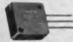
½-Inch Square Resiston Carbon Trimpot—Model 3251. Operates to 150°C / L, P, W terminals / ½ watt / 20K to 1 Meg. Sealed. Meets Mil Specs for cycling humidity.
