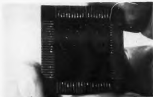
Mockup of ferrite-core logic circuit for airborne magnetic computer shows configuration that would permit storage of 400 17-bit programed words in two-hole multiaperture cores. Density is expected to reach 2,700 bits per cu in.
