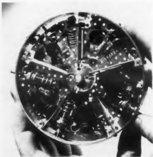
Breadboard model of 72-mc receiver in main rocket of proposed "mother-daughter" ionosphere rocket.
