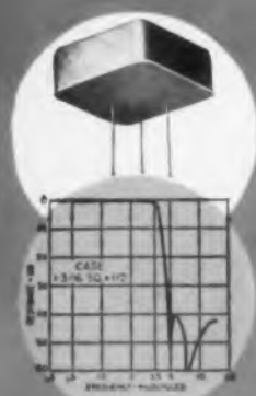
Miniaturized 3.5 KC low pass filter. 10K ohms to 10K ohms. Within 1 db up to 3500 cycles. Greater than 40 db beyond 4800 cycles.
