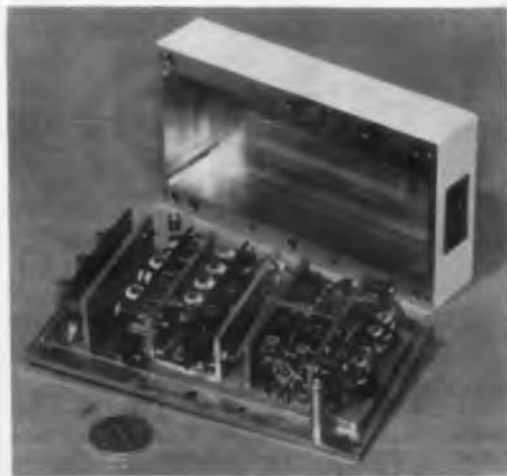
Telemetering transmitter for Navy's Transit satellite will be mounted externally. Stages, from left to right, are output filter, frequency quadrupler, power amplifier, matching network, preamplifier and frequency doubler, and first rf amplifier.
