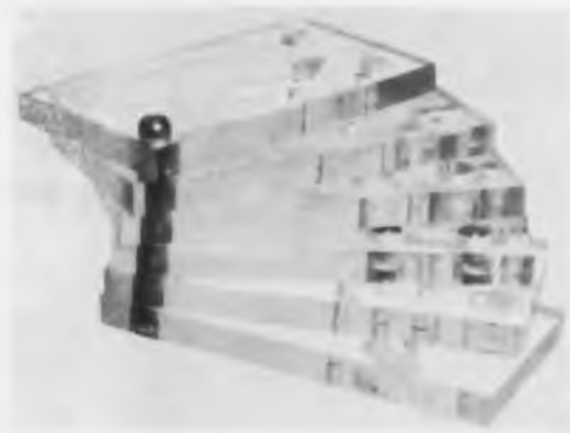
Structure of Kearfott pneumatic digital element shows how ball valves fit in chamber drilled in plastic plates sandwiched between end-plates. Horizontal grooves etched in plastic permit gas flow. Electrical pickoff would be made by coils or capacitor plates imbedded in the channel walls or ends.
