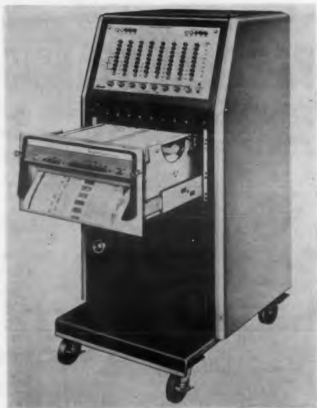
Direct-Writing Recorder 254 Accurate to 1/2%
