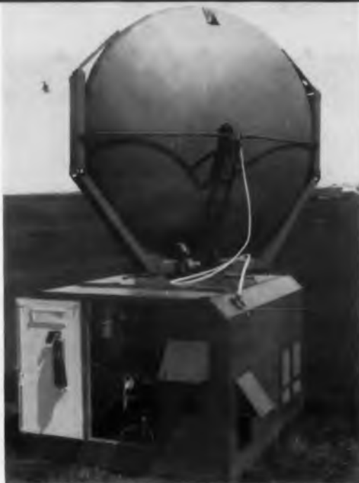
Microwave communications terminal for Pershing missile weapon system is air transportable and completely contained in 65-in. high shelter. Range is up to 100 miles via tropospheric scatter. Antenna is inflatable, aluminum-coated plastic.
