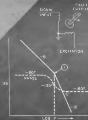
Fig. 3. Servomotor's corner (1) is important because it is usually the lowest frequency corner in the system and is followed (in a position servo) by a -180 deg phase shift.
