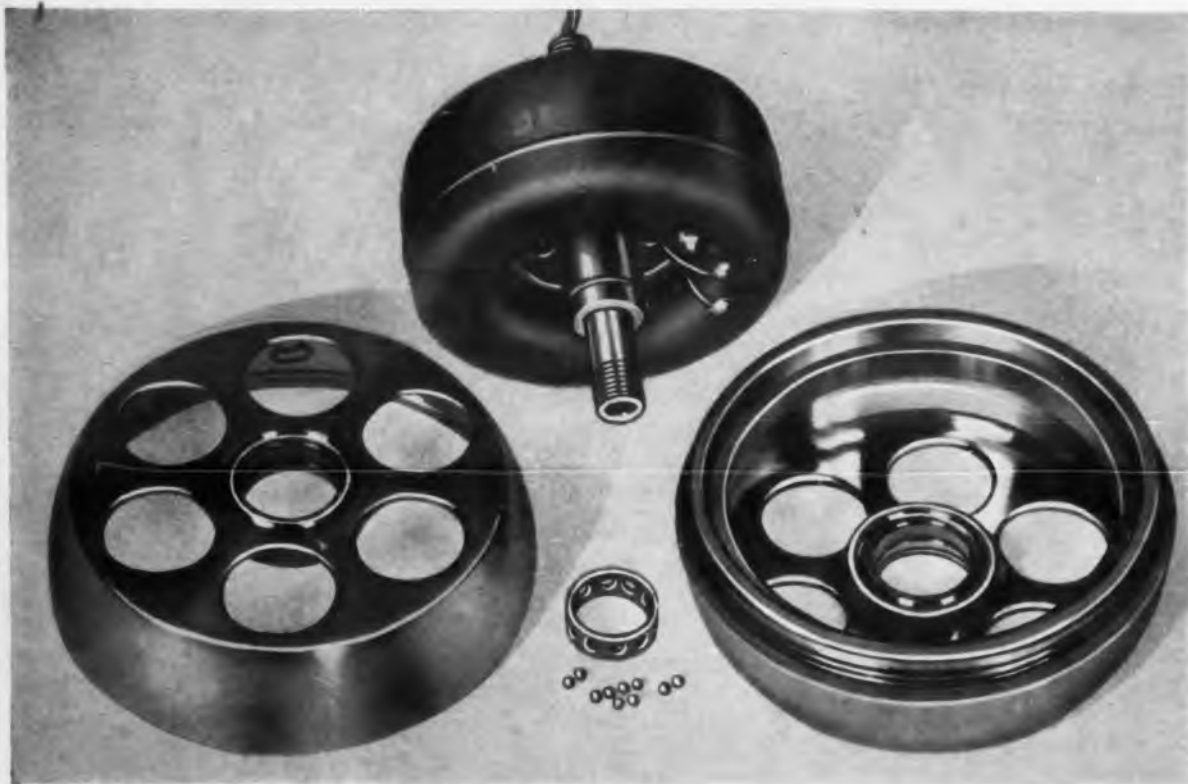
Gyro spin motor shown partially disassembled, produced by Fafnir for B-58 Hustler Bombers
