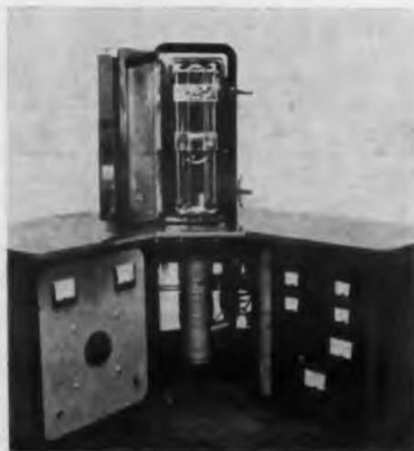
Zone-Refining Apparatus 253 Uses Electron-Beam Bombardment
