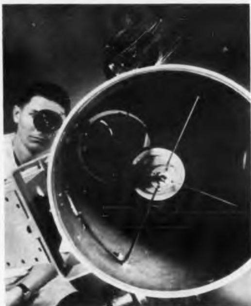
Hughes coherent light detection and ranging equipment avoids use of energy-interrupting modulator at laser output. Colidar can differentiate between two side-by-side tanks at six miles distance.
