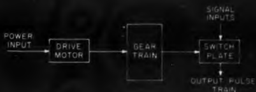
Fig. 1. Basic components of electromechanical commutator are driving motor, reduction gears, and switch plate. (Or, switch plate can be replaced by ring segments mounted on inner or outer walls of a cylinder.)
