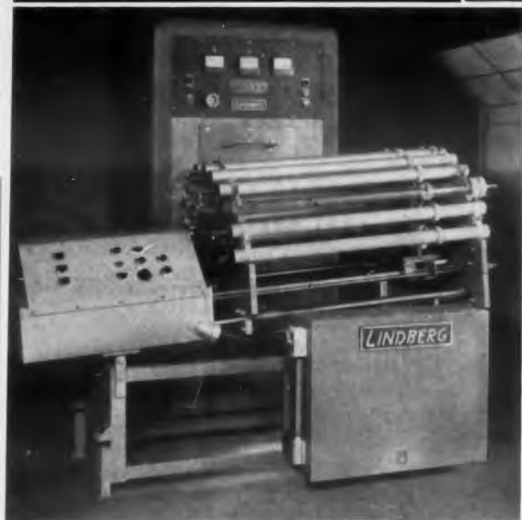
Newly-designed Lindberg Horizontal Zone Scanner provides zone purification of metallic germanium and other metallic and organic materials. Lindberg can also furnish Floating Zone Scanners for the purification of silicon.
