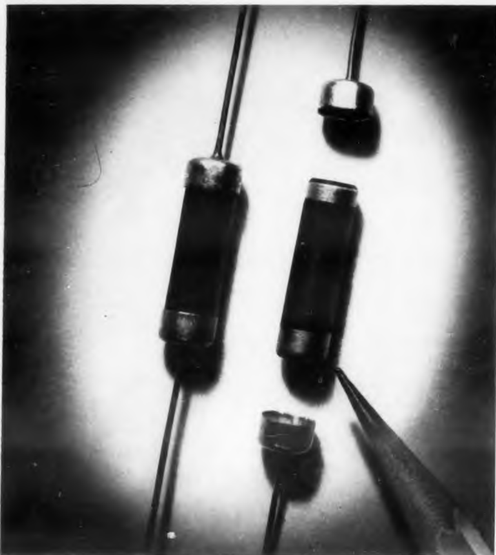
Wire leads are cemented to resistor by Du Pont thermosetting silver composition.
