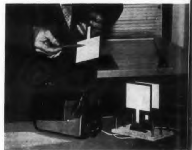
New power source consists of iron sheet coated with special enamel. Enamel is coated with thin layer of silver. Toaster was used in Westinghouse demonstration to heat the sandwich, which give high specific power both in and out of hot environment.
