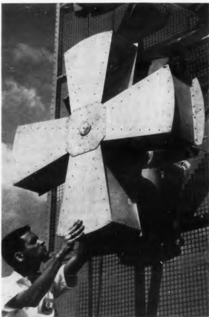
Fig. 3. This Maltese-cross Chance-Vought antenna, for service with space vehicles, functions as a vertically or horizontally polarized antenna, or as a clockwise or counterclockwise helical antenna.
