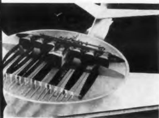
Fig. 2. One solution to the problem of large frontal area of airborne radomes is this swept-volume efficiency (SVE) antenna of GB Electronics, based on multiple end-fire-array principle.
