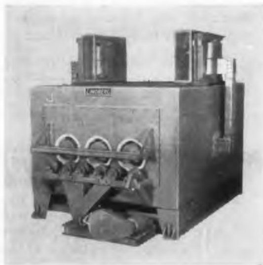
Lindberg Three-Tube Electric Rotary Calciner for calcining ferrite powders. This model is equipped with Lindberg CORRATHERM heating elements. Lindberg Calciners can be supplied with either fused quartz or alloy tubes. When required, gas-fired models are also available.
