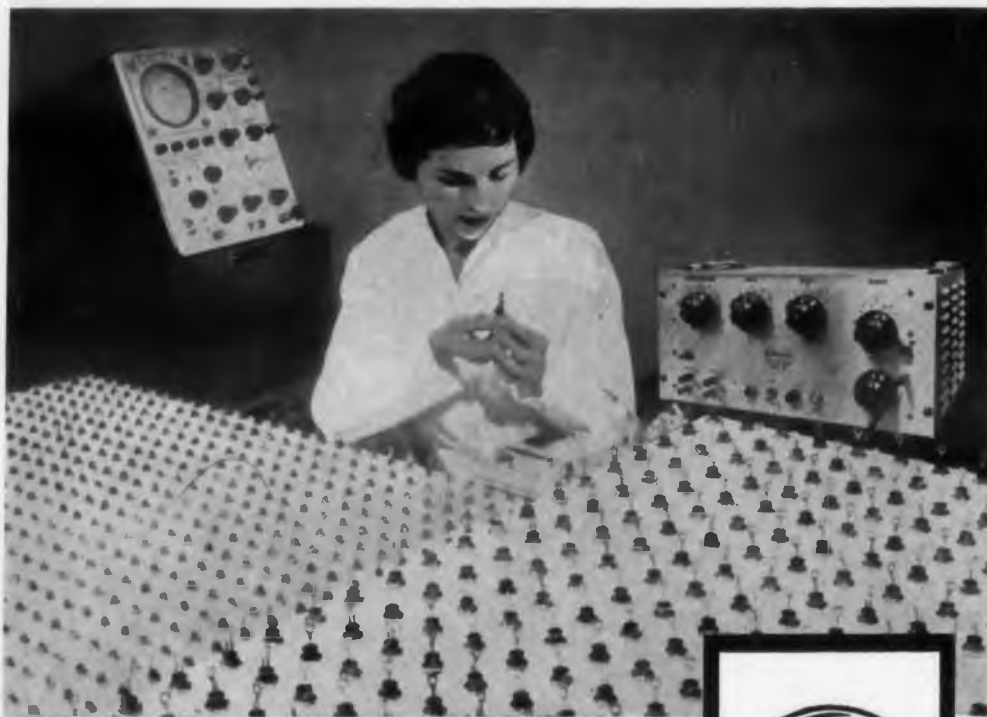
"A Rutherford pulse generator is being used to test silicon rectifiers at the Clyde, N.Y., facilities of the G. E. Semiconductor Products Department."
