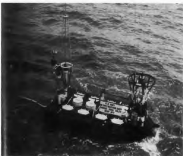
Gulf buoy which will carry the planned 30-w thermoelectric generator provided early warning of last summer's Hurricane Ethel. It transmits on 5,340 kc for 3 min every 6 hr. Use of such buoys is likely to increase as instrumentation and power sources are improved.
