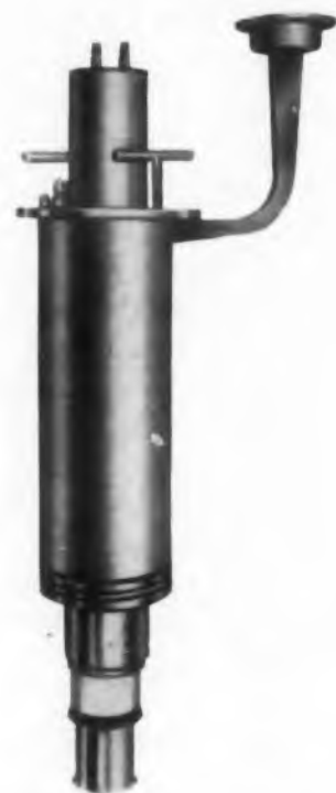
Fig. 5. Tapered slow-wave structure, used in Varian's VA-125A, makes possible 2-megawatts pulse power at over 45 per cent efficiency.
