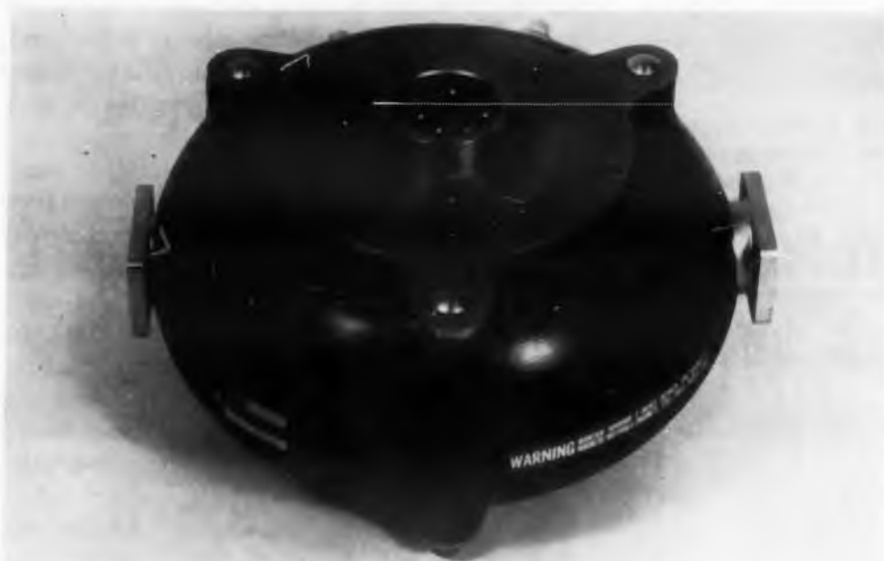
Fig. 4. Crossed-field forward-wave amplifier, type L-3280, developed by Litton, preserves magnetron efficiency without usually attendant frequency instability.
