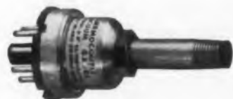
VTP 6343 THERMOCOUPLE GAUGE TUBE Fast response: less than 0.1 second! Pressure range: 0.1 to 1000 microns. Ruggedized all-metal construction. Useable for leak detection on vacuum systems as well as absolute pressure measurement.
