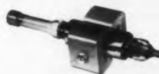
VTP PG-7 PHILIPS GAUGE Small, compact, stainless steel gauge. Measures to 10 -9 mm Hg. Withstands 425° bakeout temperatures. Easily cleaned. Leak-free. Adaptable to any vacuum system. Sputter shield for long service life.
