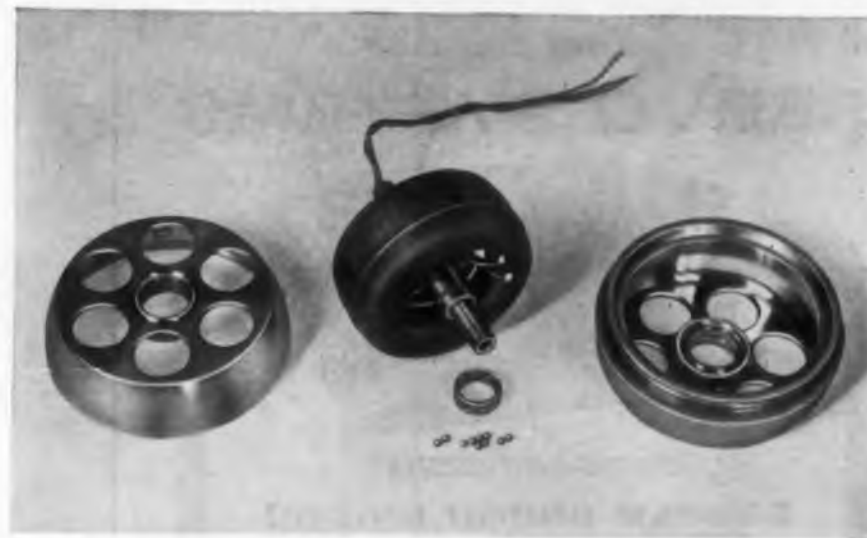
Gyro spin motor produced by Fafnir for the B-58 Hustler bomber. Fafnir super-precision ball bearings have inner races ground on the shaft, and outer races in the motor housing.
