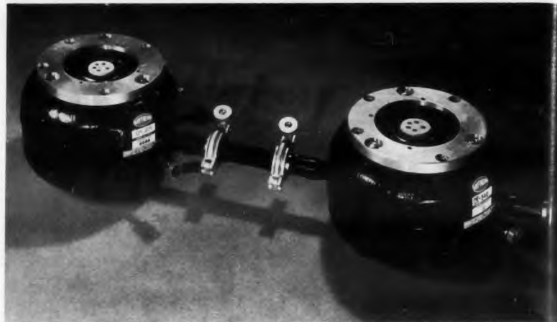
S-band Bitermitron coupled to a conventional cross-field backward wave oscillator, showing the similarity between the structure of the two tubes. In this configuration the two-terminal Bitermitron is used as an amplifier.
