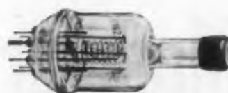
VTP 7169 IONIZATION GAUGE TUBE All glass. Designed for use in glass vacuum systems. Electrically identical to VTP 6578. Both may be outgassed easily by passing heater current through grid structure.
