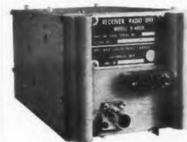
MODEL R-400A UHF RECEIVER 260 MC—400 MC 6.8" L. x 3.5" W. x 3.1" H.
