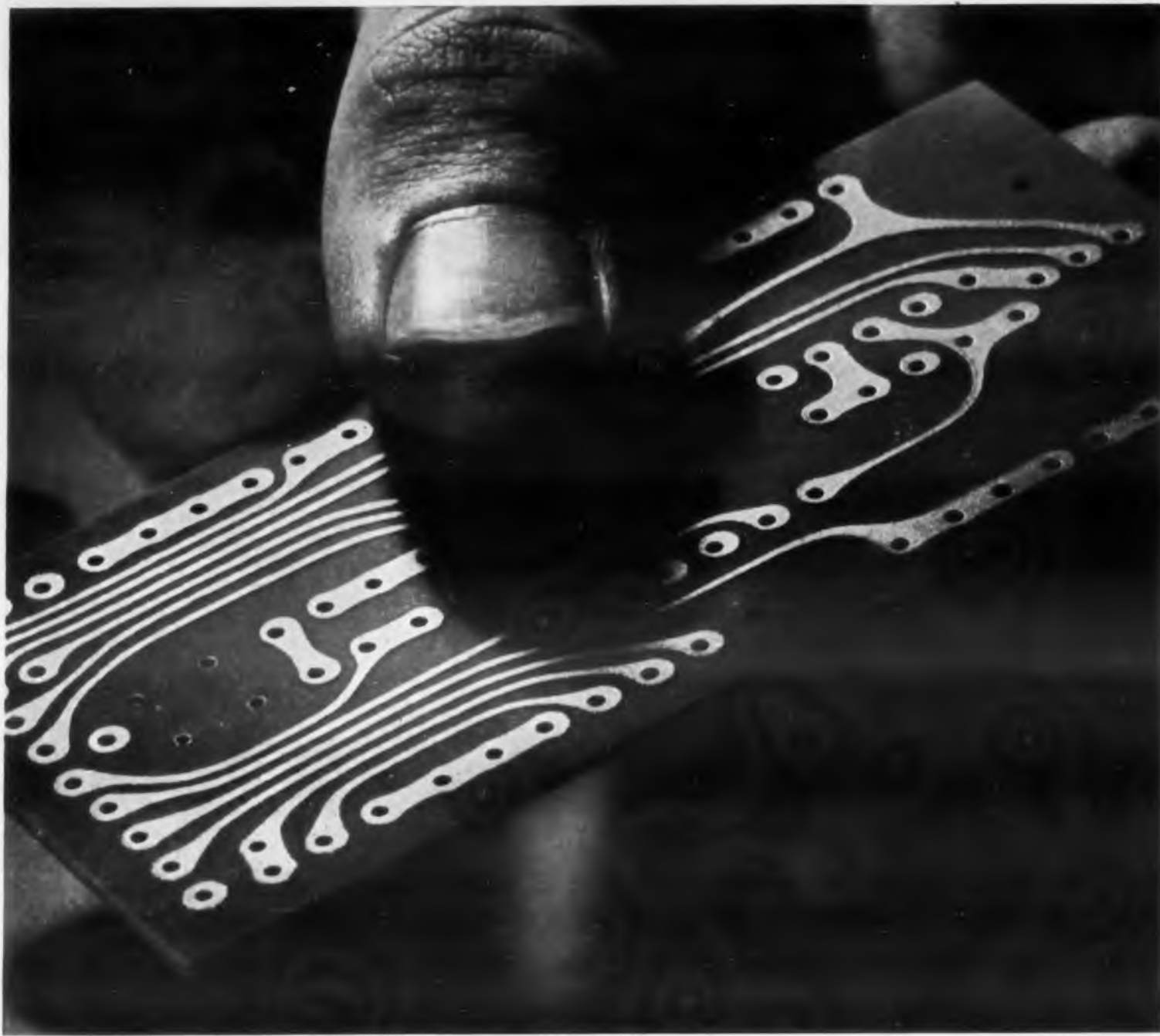
FOTOCERAM circuit board blanks are made using the micro-accuracy of photography. All holes and shapes are produced by simple exposure to light, heat, and an etching operation.
