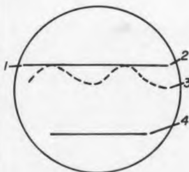
Fig. 2. The level line 1-2 of the calibrated attenuator is lined up with the ferrite characteristic, 3, traced on an overlay.
