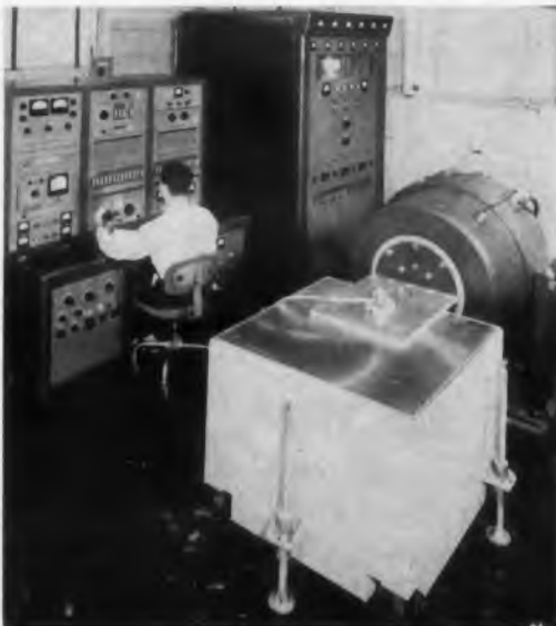
The Ling analyzer-equalizer system installed at the Rototest Laboratories consists of four major units: control console, amplifier, shaker and oil table.
