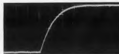
Response to a current step of 10^{-12} amp. Input capacity is 35 \mu f. One major horizontal division equals 200 milliseconds.
