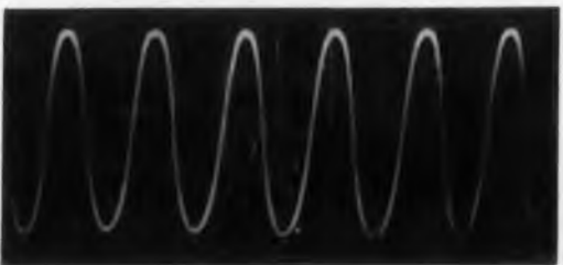
Same scope, using a sampling converter and trigger-rate converter shows clean sine wave at 300 mc.
