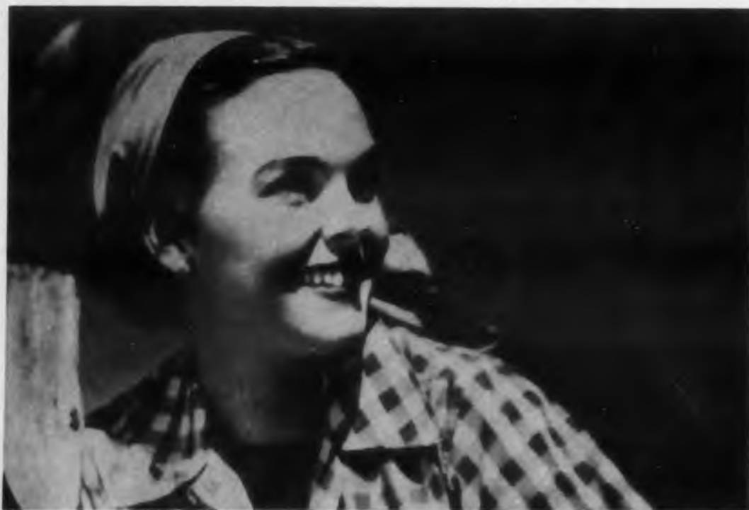
Fig. 7. Television picture transmitted using a four-digit binary code. Note the higher picture quality compared to Fig. 6.
