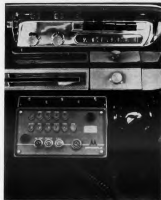
Fig. 3. One type of a pushbutton control head that is now in mobile service.
