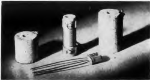
Fig. 2. High temperature wirewound resistor is shown before and after embedment in Eccoceram SM-25. In use, the imbedded unit melted internally without any adverse effect on the ceramic encapsulant.
