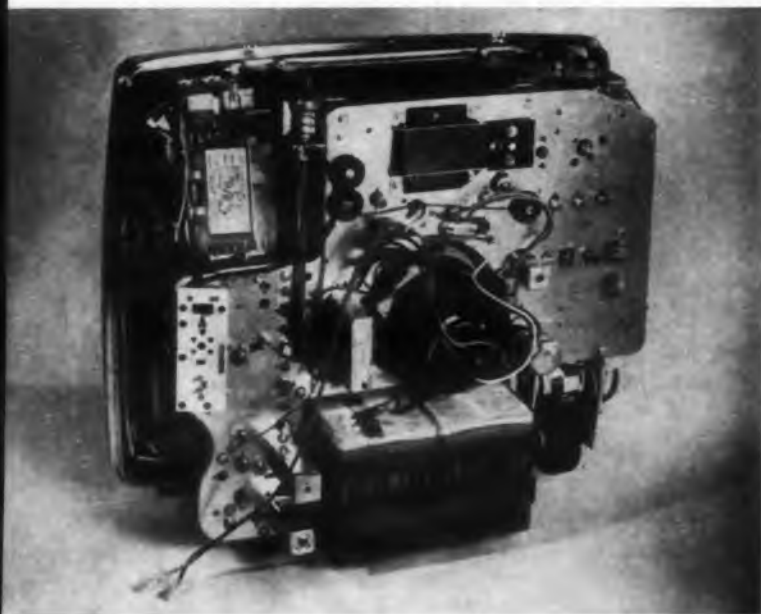
Thirty-watts (20-v, 1.5-amp) input power is supplied by the silver cadmium energy cell shown mounted in the lower center of the chassis. An average of five to six hours viewing time is claimed before recharging is necessary; a minimum of 500 recharges can be expected.
