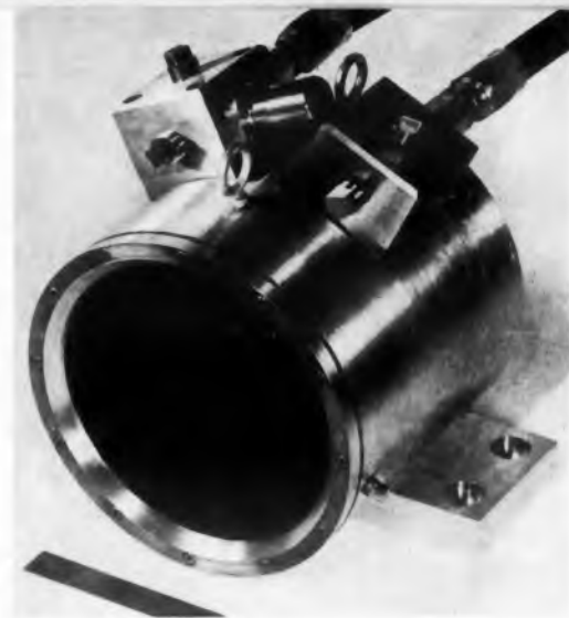
This hydroacoustic transducer , developed by Stromberg-Carlson, may represent a breakthrough. The unit, using high-pressure fluid flow to produce high-level acoustic energy, needs no costly electronic driver. A somewhat similar unit of 10 times the power, is reported by Textron's MB Electronics.
