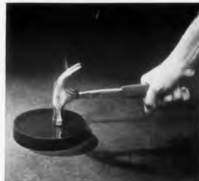
"SCOTCHCAST" Brand Flexible Epoxy Resin is subjected to full force or hammer blow with no evidence of cracking or shattering. "SCOTCHCAST" resiliency is built into resin molecule, allowing it to withstand extreme shocks permanently.
