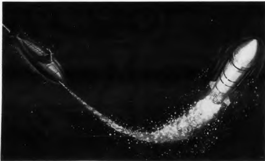
SUBROC weapon , in design by Goodyear-Kearfott team, is launched from torpedo tube to break surface for a nearly 100-mi flight and to re-enter water as a homing torpedo.
