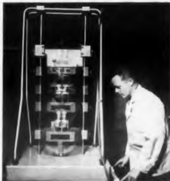
Honeywell accelerometers undergo a saw-tooth shock force of 100 G's for six milliseconds during test at the Environmental Test Laboratory of Avco's Research and Advanced Development Division.
