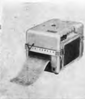
Recent Models of the 906 Visicorder incorporate time lines and grid lines and record up to 14 simultaneous channels of data.
