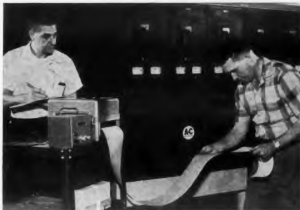
N. O. Risch and F. R. Manning, design engineers at Allis-Chalmers Norwood Works, study a Visicorder chart of voltage-drop tests on a generator.
