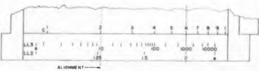
Fig. 2. For Power Ratios: — 1 on C scale is aligned with 10 on LL3 scale.
