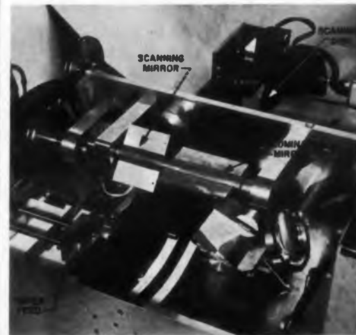
Business end of Air Force page reader. Scanning and illuminating mirrors on common shaft oscillate across the width of the page to be read. Paper is curved to provide equally long optical path at every point.
