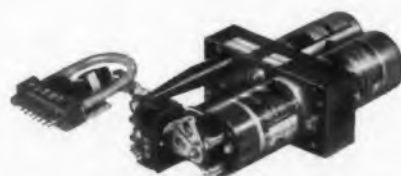
SERVO ASSEMBLY - Type 9 motor generator driving two Type 11 CT synchros through a slip clutch and a gear train having ratio of 1500 to 1.
