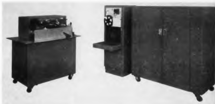
Prototype page reader developed for Air Force is housed in three cabinets. Scanning equipment is at left. Center cabinet contains tape punch, and cabinet at right houses logic and addressing equipment. Commercial models will be transistorized and fitted into one cabinet.
