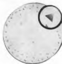
Dislocation density, Knapic silicon monocrystals grown by a modified Czochralski technique: Crystal diameter to 3/4" — None; 3/8" to 3/4" — less than 10 per sq. cm.; 1/4" to 3/8" — less than 100 per sq. cm.; 1/8" to 2" — less than 1000 per sq. cm.
