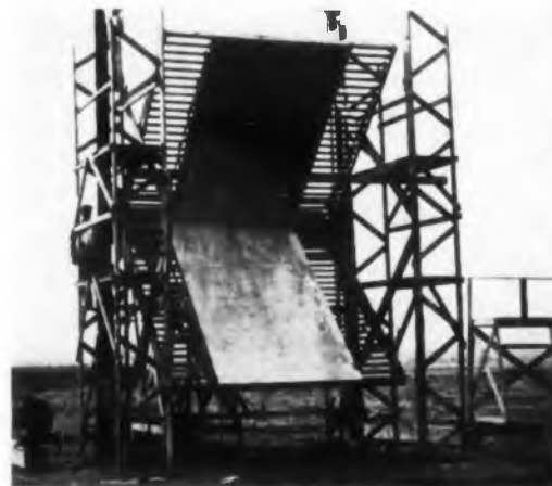
Fig. 1. Experimental corner-reflector antenna analyzed by the National Bureau of Standards. Length and width of reflecting surfaces, position of dipole, and aperture can all be varied to determine effect on gain.
