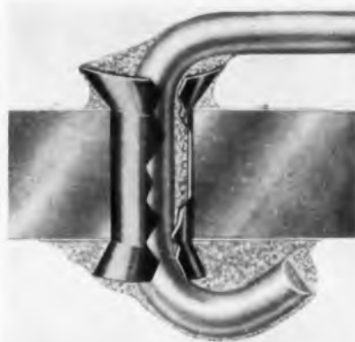
Enlarged cross section of United Funnel Flange Eyelet showing greater soldered area which lends greater strength.
