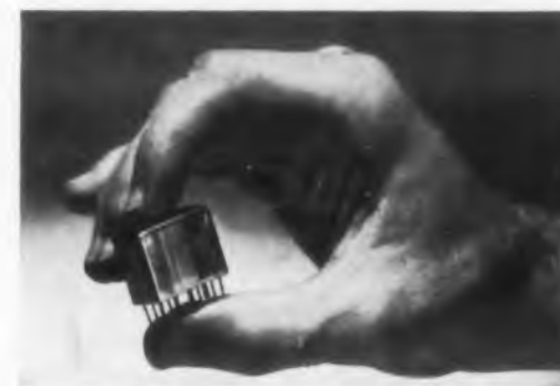
4-Pole micro-miniature suited for 160C ambient
