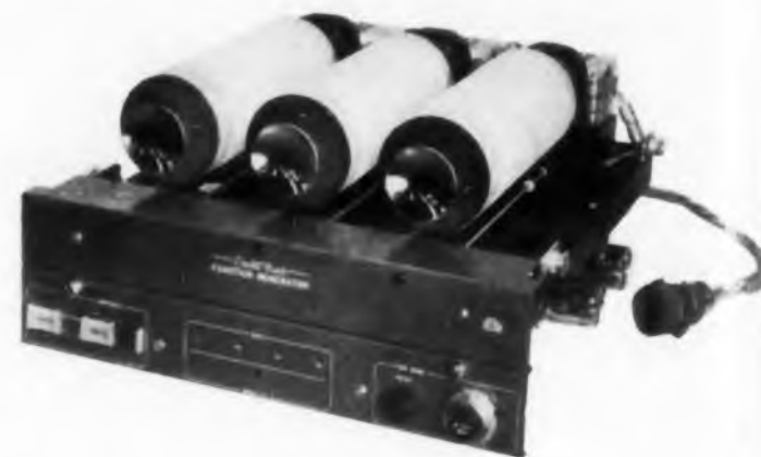
Three-channel function generator (with case removed) reads three charts on separate drums.
