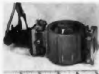
Stabilization Cavity For 8500 to 9600 mc frequencies
