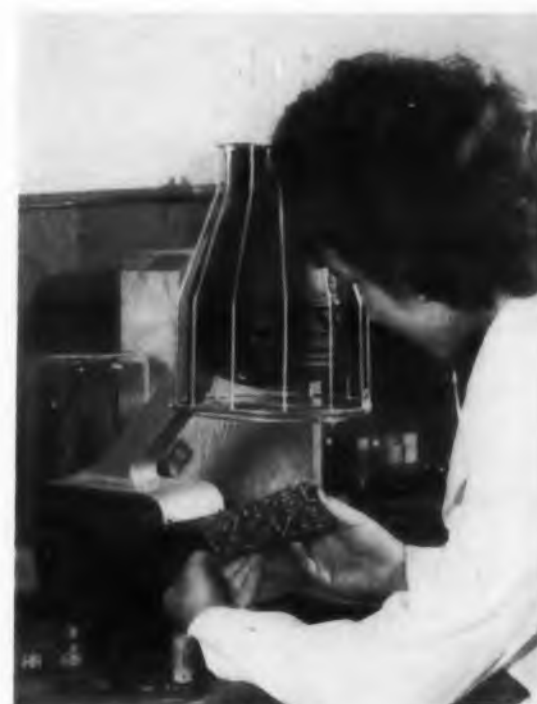
Residual solder flux, almost invisible in ordinary light, glows brightly under the Blak-Ray.
