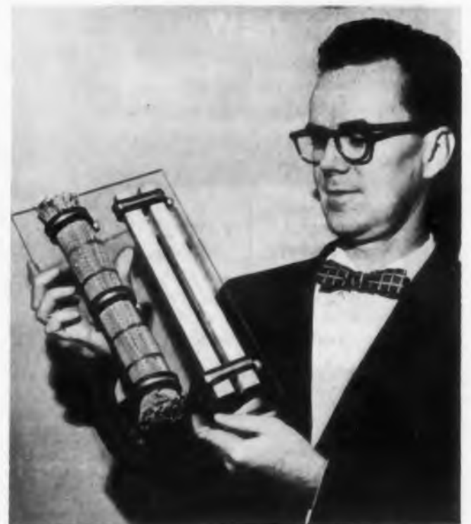
Two rigid, fiber glassed sections hold about the same number of wires as conventional harness.
