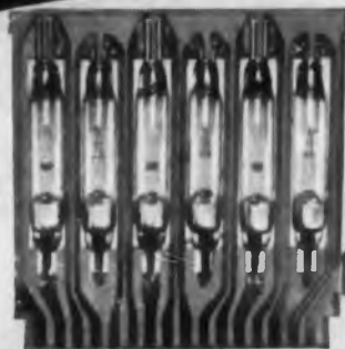
Arrangement of six-in-line mercury-wetted contact switches on printed circuit panel.
