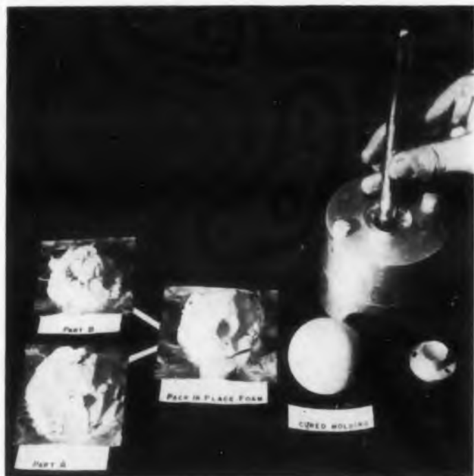
Fig. 2. Ingredients and finished molded piece, resulting from a "pack-in-place" procedure.
