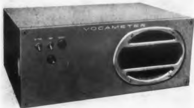
Girl's voice calls out measurements made by this voltmeter. Unit has a 14 word vocabulary.
