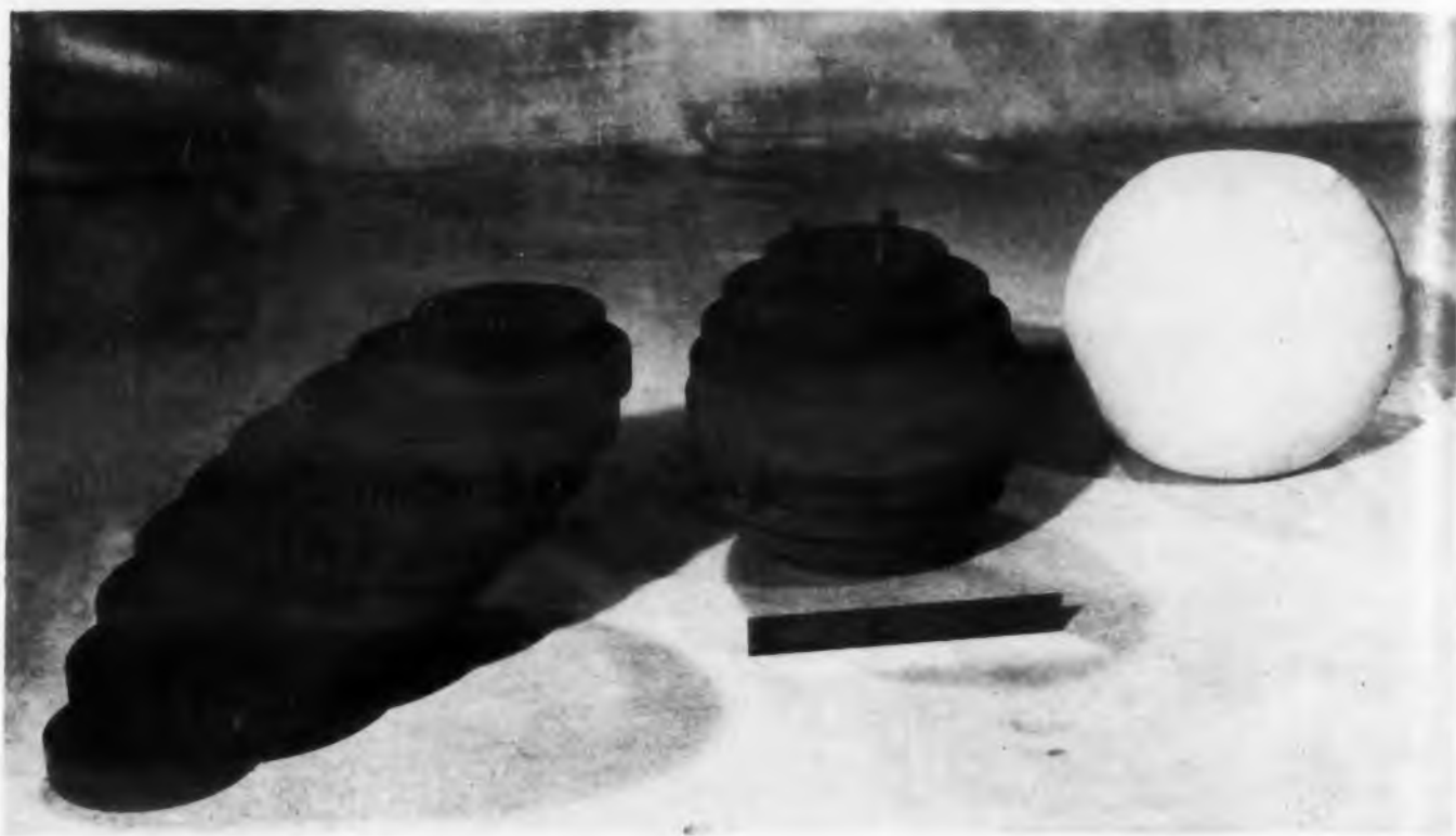
Fig. 3. Disks and a sphere are typical shapes fabricated from glass microballoons.
