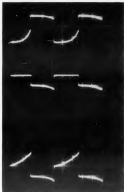
Fig. 1. Typical transistor multivibrator circuit with collector voltage waveform.
