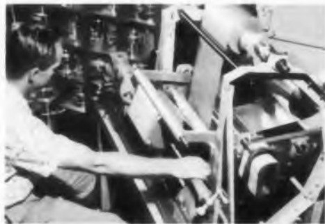
Interleaving sheet-type insulation with aluminum strip.
