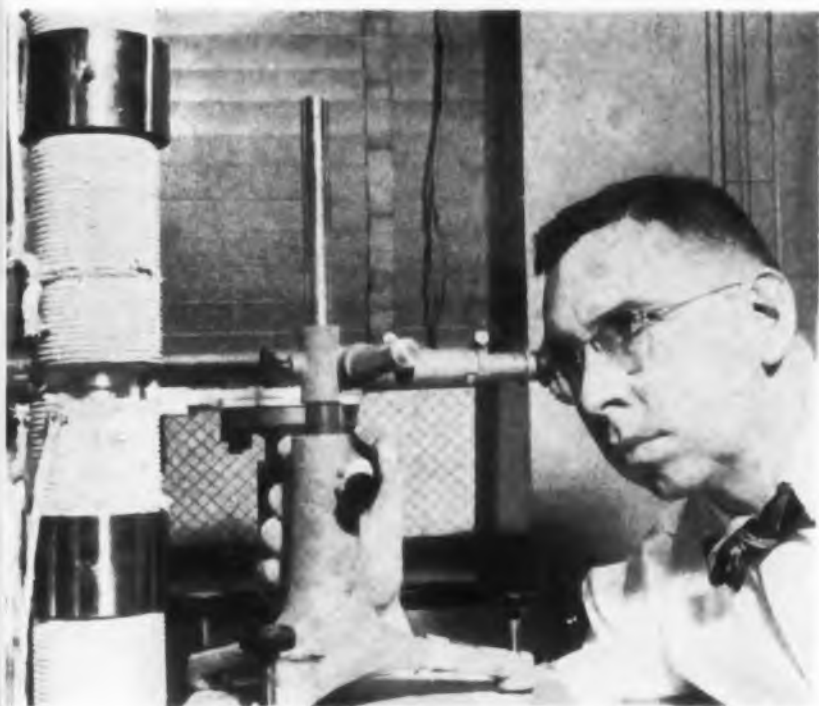
Crystal growing equipment used in Bell Labs' floating zone process. Molten zone of a gallium arsenide rod is examined during crystal growing experiment.
