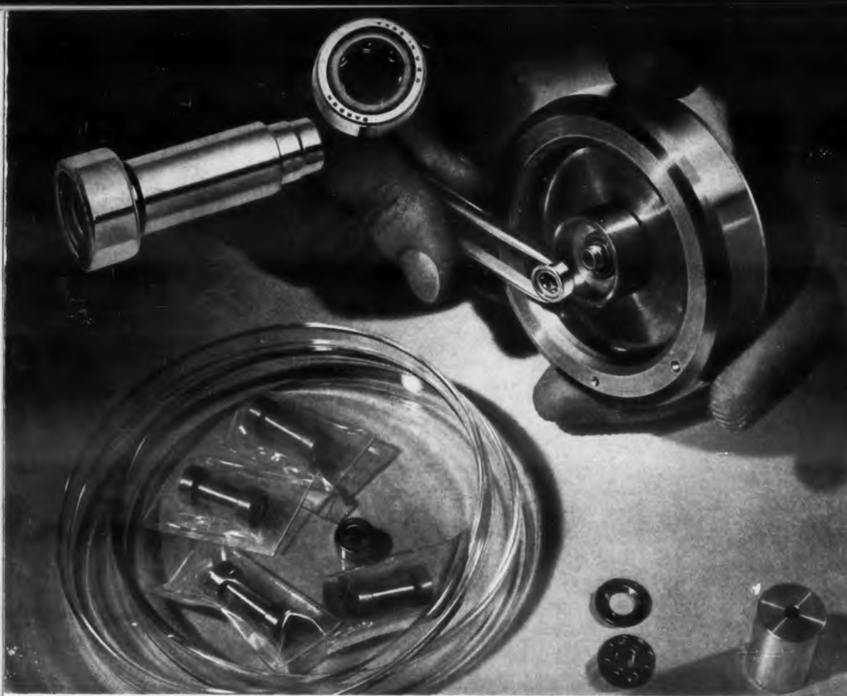
Barden Precision Z148 bearings specially designed for a gyro rotor
