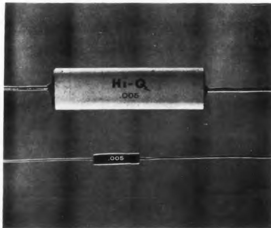
Fig. 1. A paper capacitor (top) vs a Cerafil capacitor (bottom).
