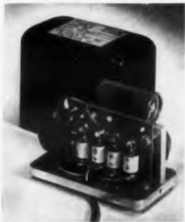
DC to DC Converter 300 v dc output
