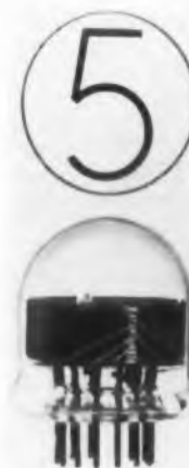
Fig. 2. Display units combining several projection systems in horizontal rows. Manufactured by Industrial Electronic Engineers, North Hollywood, Calif.
