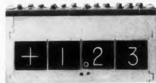
Fig. 1. This edge-lighted display is manufactured by Non-Linear Systems, Inc., Del Mar, Calif. Lighting both numeral and the decimal point simultaneously provides a combination of two symbols.
