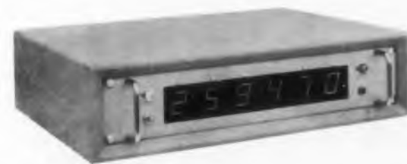
Fig. 5. Seven lighted characters form the numerals 0 through 9 in this unit, manufactured by Beckman Instruments Inc., Berkeley Div., Richmond, Calif.
