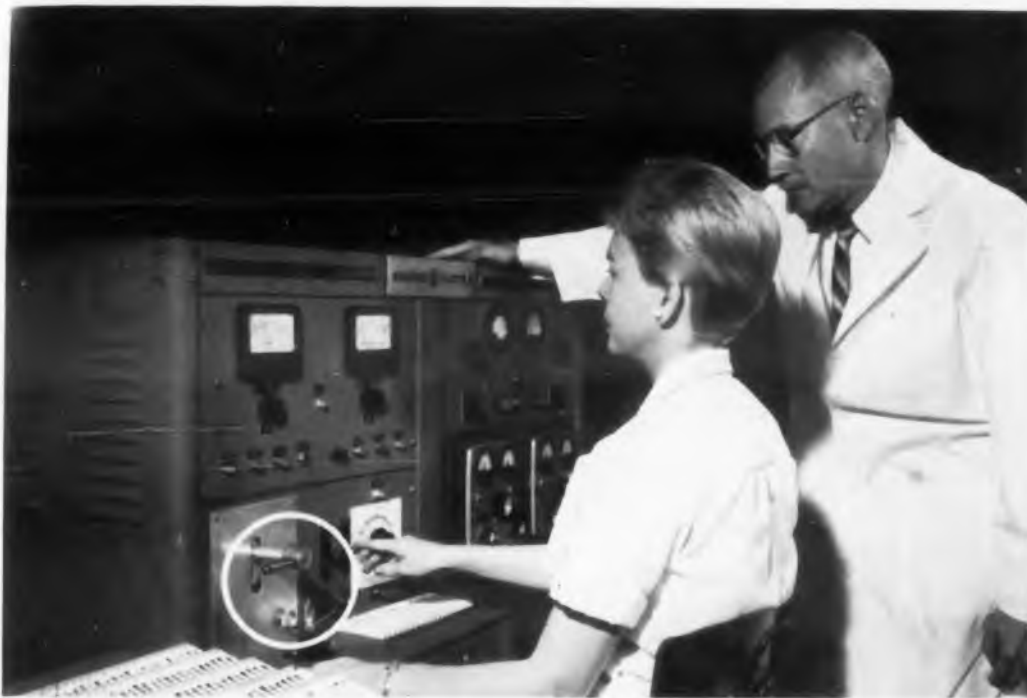
IMPULSE-TESTING G-E SUBMINIATURES. R. W. Field, Manager, Finished Tube Quality Control, General Electric Owensboro tube plants, watches test operator take peak and integrated output readings as 5-Star 6111's are tapped by pendulum (circle). To assure accurate readings, the meter pointers remain in indicating position until operator presses the reset button.
