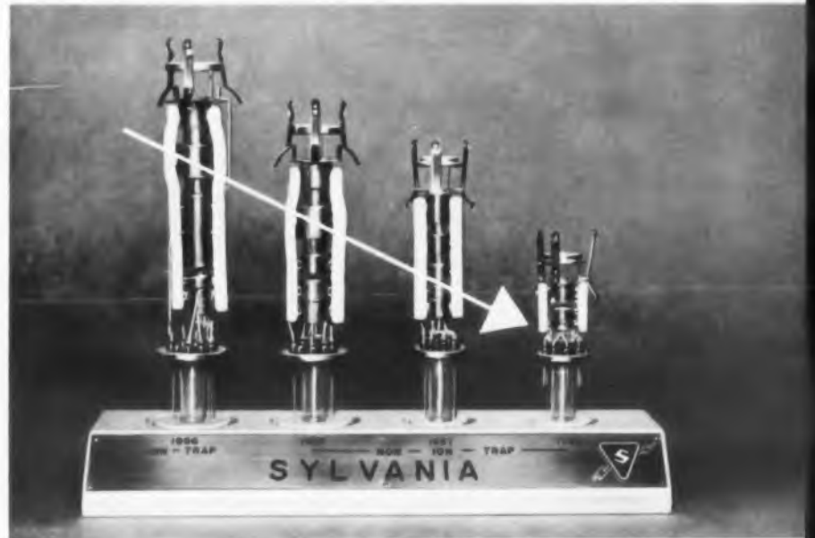
Tripotential Electron gun is a major advance in the evolution of shorter television picture tubes
