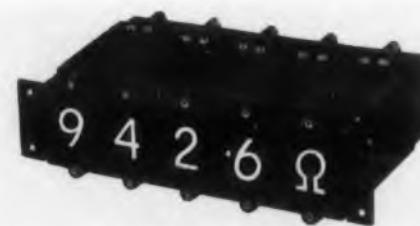
Fig. 2. Display units combining several projection systems in horizontal rows. Manufactured by Industrial Electronic Engineers, North Hollywood, Calif.
