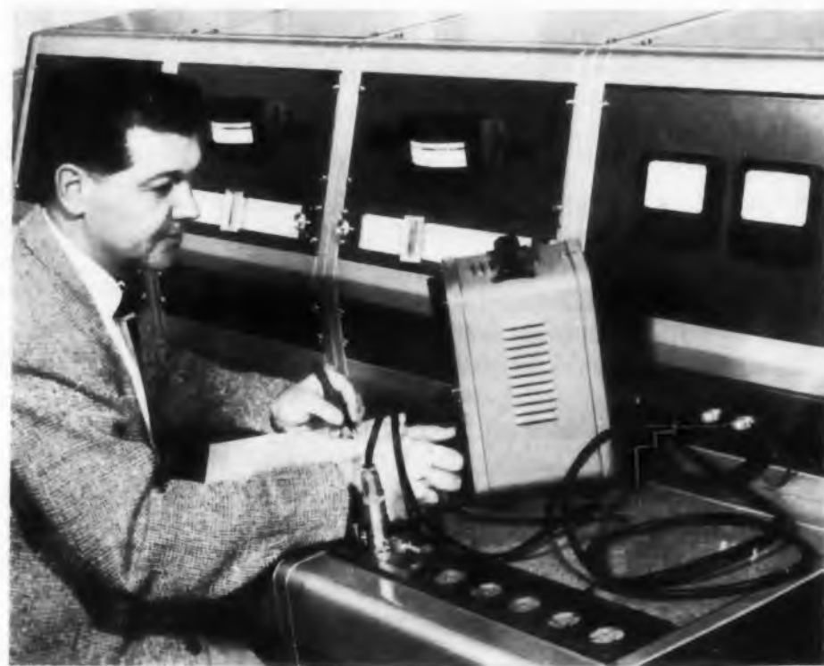
RF calibration consoles of the type used in the calibration of voltmeters.
