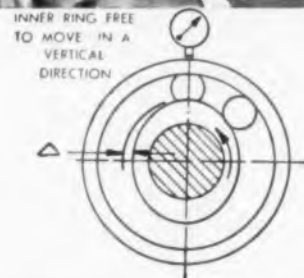
Fig. 2 — Inner raceway is out-of-round, although concentric with bore.
