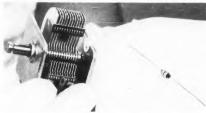
The tiny Varicap unit shown on the right has replaced the tuning capacitor in an experimental standard broadcast receiver. It has also replaced an afc vacuum tube circuit in an fm tuner.
