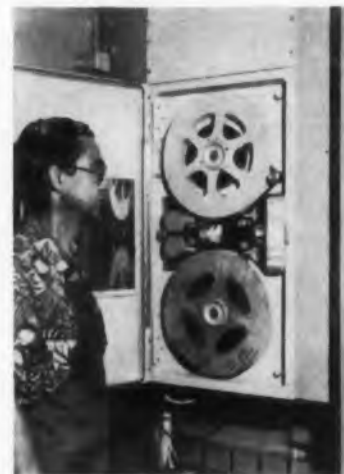
Control tape on an Ampex FR-100 can hold over 1 million commands for each axis of tool movement
