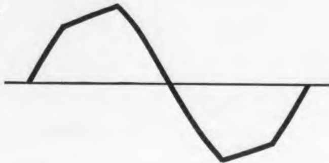
Fig. 4. Phase shift is responsible for diagonal clipping.
