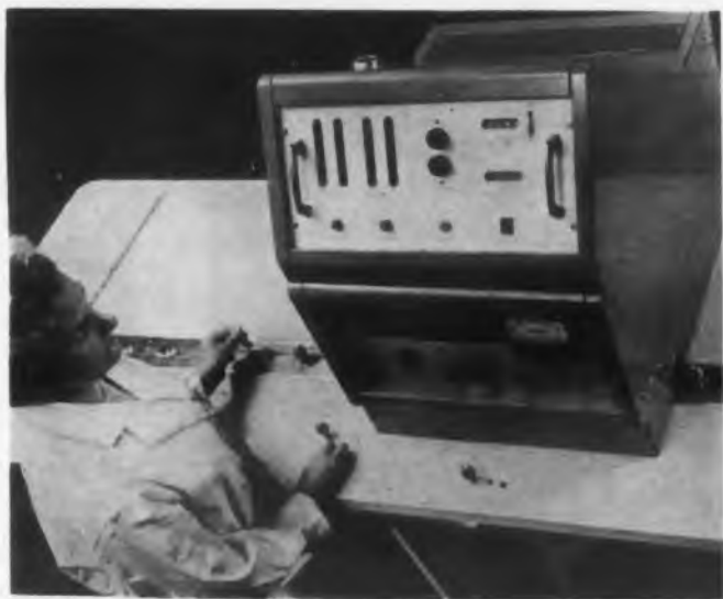
Atomonitor inspects production-line assemblies for the presence of hidden vital parts.
