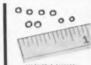
MAGNETIC MEMORY CORES AND PLANES
