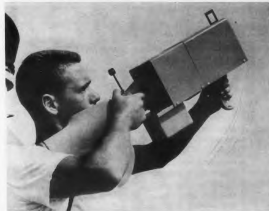
Radiometer is one of the instruments used to measure the radiation from the Jupiter IRBM as it re-entered the atmosphere.
