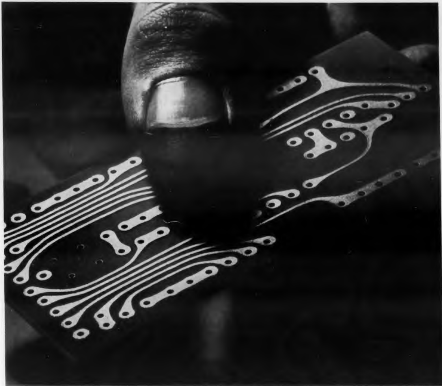
FOTOCERAM circuit board blanks are made photographically. All holes and shapes are produced by simple exposure to light, heat, and an etching operation.
