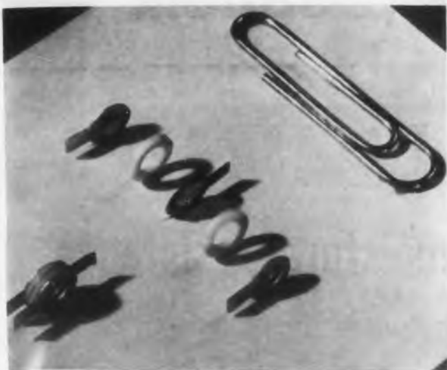
Inside view of GE's new no-filament high-temperature tube.
