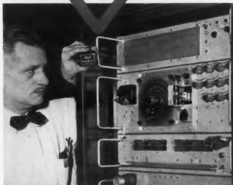
Automatic Electric Polar Relay is used in selector cabinet of Tele-register Corp. stock-quotation system. Teleregister design engineer, Jim Hartelius, shows how snap-on cover can be removed for visual inspection. He reports "... complete reliability ... almost infinite life ... virtually never gets out of adjustment."
