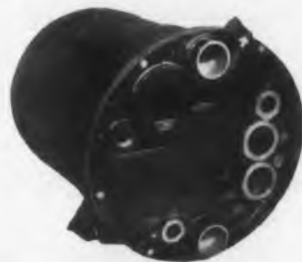
Electronic guidance equipment mounted to both sides of UAP cold plate, contained in UAP pressurized case... for control of air-to-air missile.
