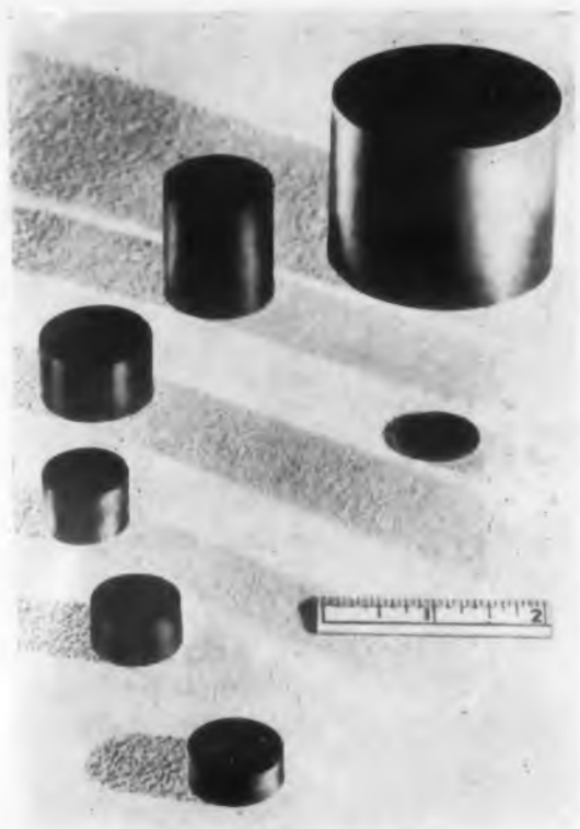
Off-the-shelf samples of yttrium-iron garnet, a rare earth expected to replace ferrites in microwave applications.
