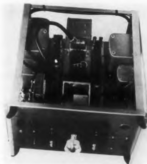
Fig. 3. The assembly mounts in a standard 19 in. chassis containing all necessary power supplies.
