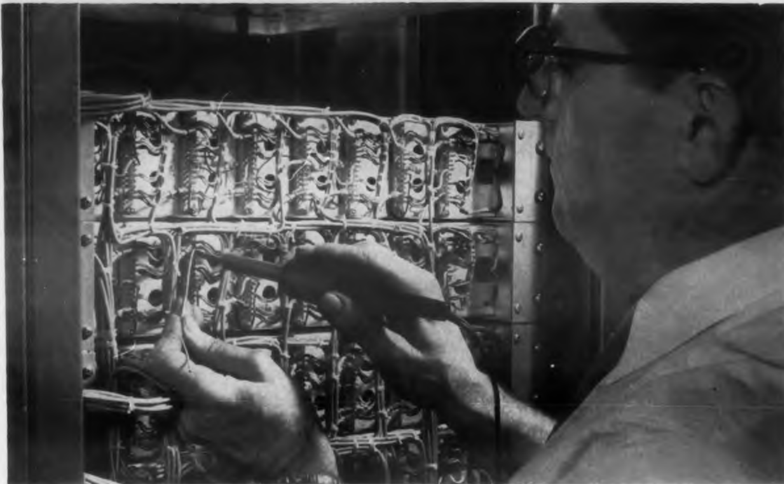
In hundreds of applications, such as this computer, R/M "Teflon" tape-covered wire offers the ultimate in dielectric strength and trouble-free performance.
