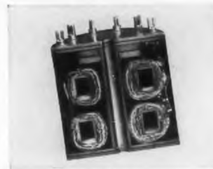
Section of magnetic amplifier coils embedded in Epon resin by Westinghouse Electric Corporation, Pittsburgh, Pa.
