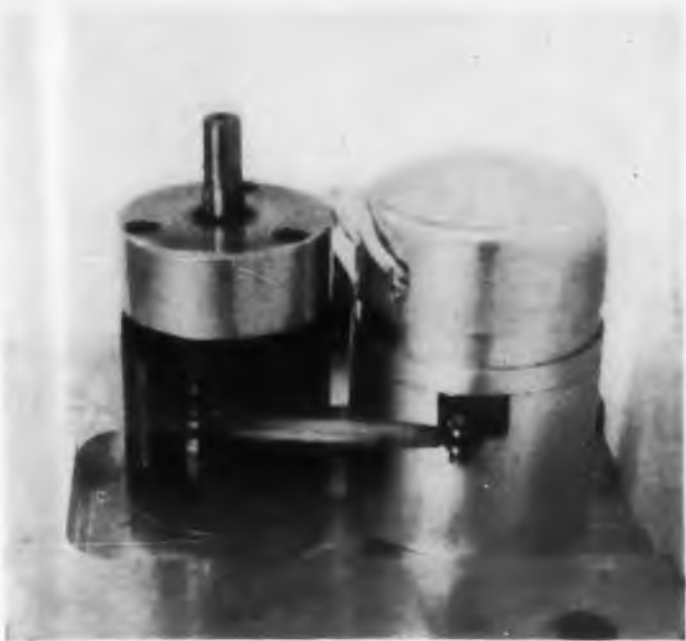
Mechanical clutch (left) and electrical transducer (right) mounted on servo breadboard plate.
