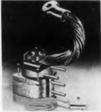
670 Amp Power Junction 9.8 Per Cent Efficiency
