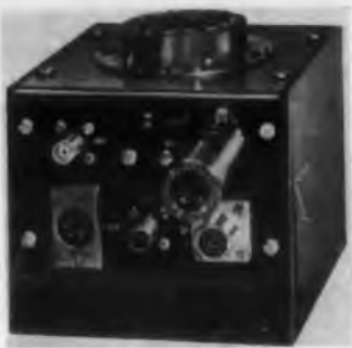
Photomultiplier Preamplifier For Driving Long Coax Cables
