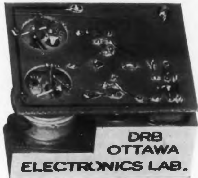
Fig. 5. The complete servo amplifier unit.
