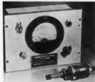
Vacuum Gages Thermocouple and Ionization Types
