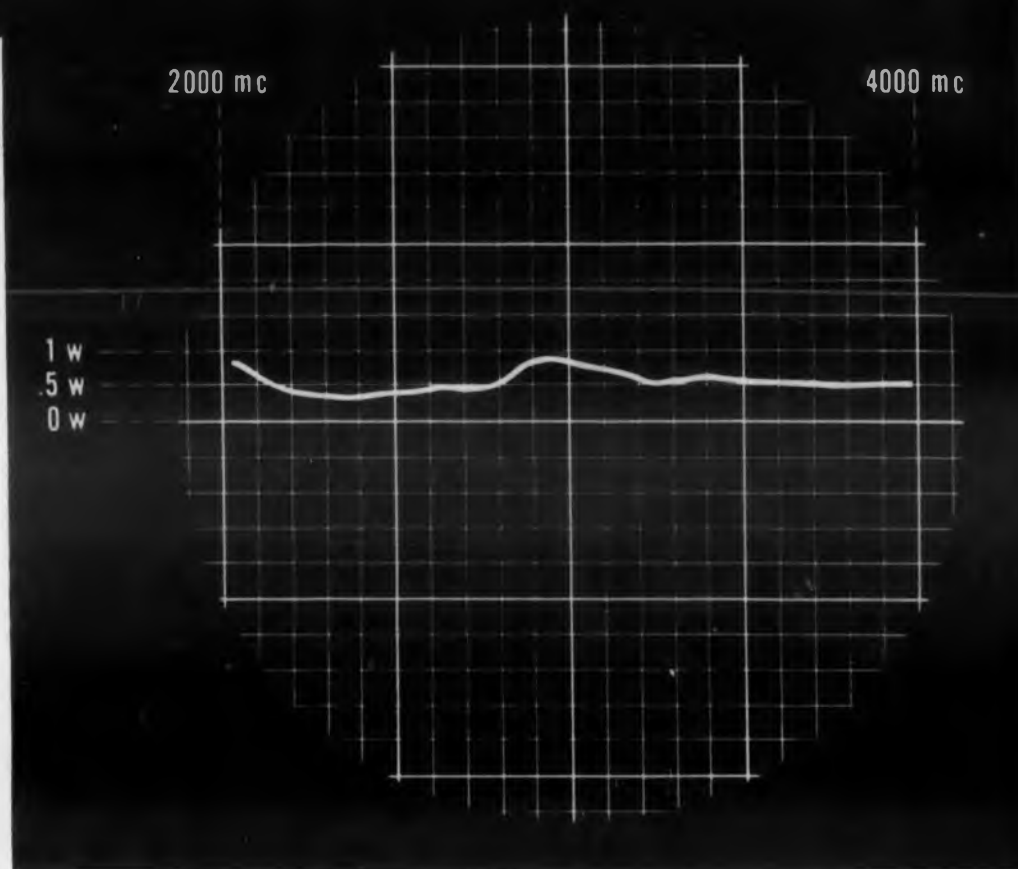
▲ Observe from the scope presentation above (actual photograph made with a production GL-6917 on test) how power over the entire 2000-mc tuning range is substantially constant, varying only .5 w. Because tube frequency, with voltage-tunable magnetrons, is a linear function of anode voltage, an r-f signal can be tuned at will to any frequency in a wide spectrum.
