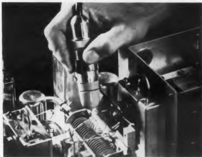
Fig. 2. Practical application of irradiated polyethylene in VTVM test probe.
