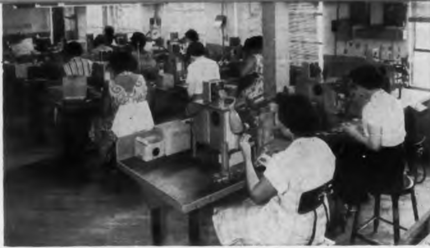
Ample Production Capacity —In this corner of the Assembly Department, spot-welding operations are performed on relay and thermostat sub-assemblies.
