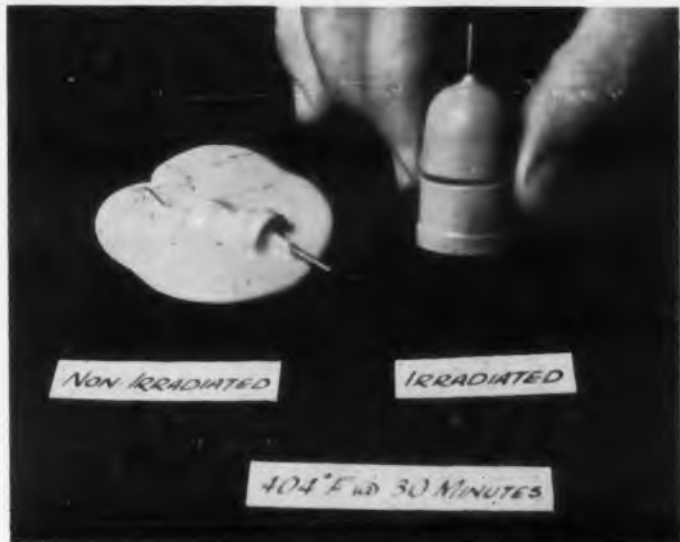
Fig. 1. Effect of irradiation on polyethylene at high temperature.
