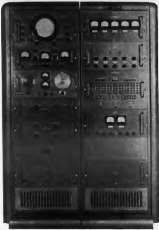
Fig. 1. Typical electronic equipment forced-air cooler. Blowers at bottom of cabinet bring air in through filters and force it out through top of cabinet.
