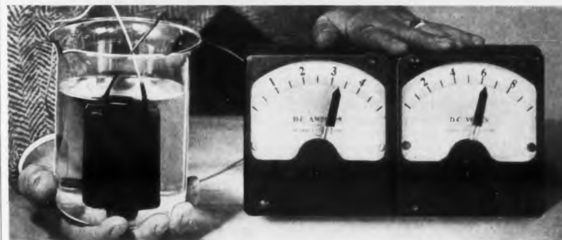
POWER These silver-chloride/magnesium type batteries deliver up to 42 watt hours per pound and 3 watt hours per cubic inch, with nearly level power output over total operating life.
