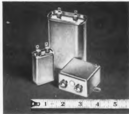
PERMAFIL RECTANGULAR solid dielectric in case styles CP50, CP60, and CP70 series. Built to electrical requirements of characteristic "K", MIL-C-25A. Ratings: .01 uf to 10 uf; 100 v. d-c to 1500 v. d-c, Temp. range: -55C to +125C.
