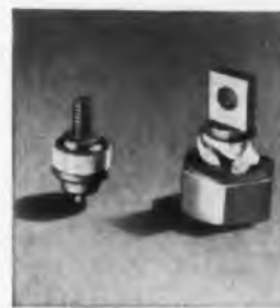
Right—Sample of a Stupakoff Alumina Terminal in test rig, torsion-tested to destruction. The failure occurred in the ceramic, not in the bond.
