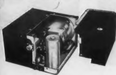
MODEL E/MT-200, TYPE 201 DISSIPATION: 1,000 watts. ALTITUDE RANGE: sea level to 50,000 feet. POWER REQUIRED: 28 volts D.C. WEIGHT: 14 1/2 pounds. SIZE: 10" x 10" x 6" high.
