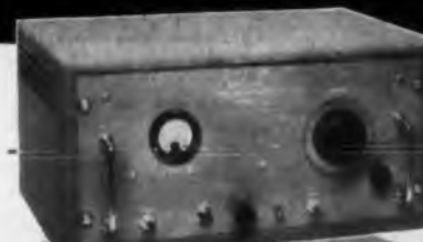
Model 5585 Selective Amplifier provides 100 microvolt sensitivity in the 0-42 mc range. Price, $425.00
