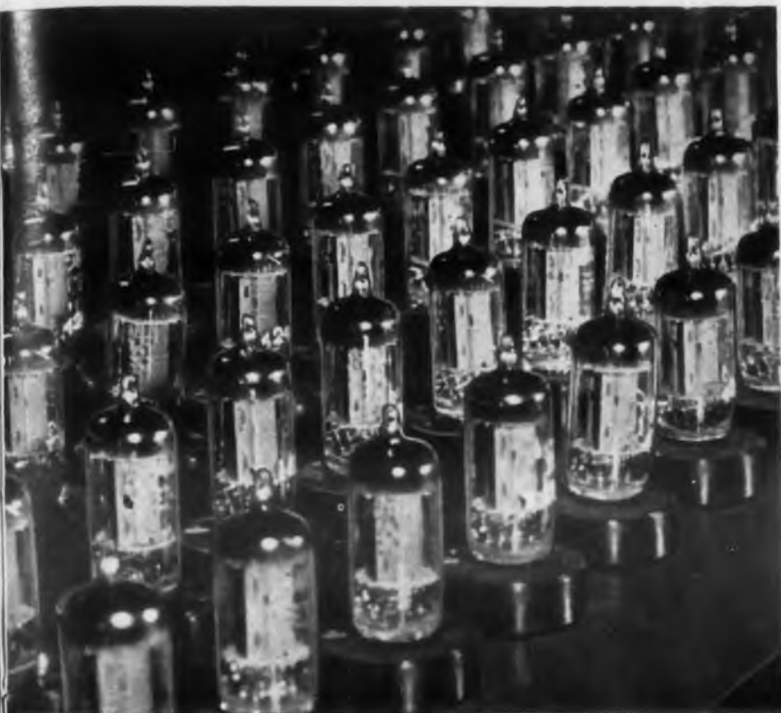
▲ SPECIALLY TESTED . . . BIASED TO CUT-OFF FOR LONG INTERVALS! Life tests of G-E computer tubes under cut-off conditions, are made in order to be sure no "sleeping sickness", or failure to respond to grid input pulses, develops during inactivity. This is determined by means of periodic interface checks.
