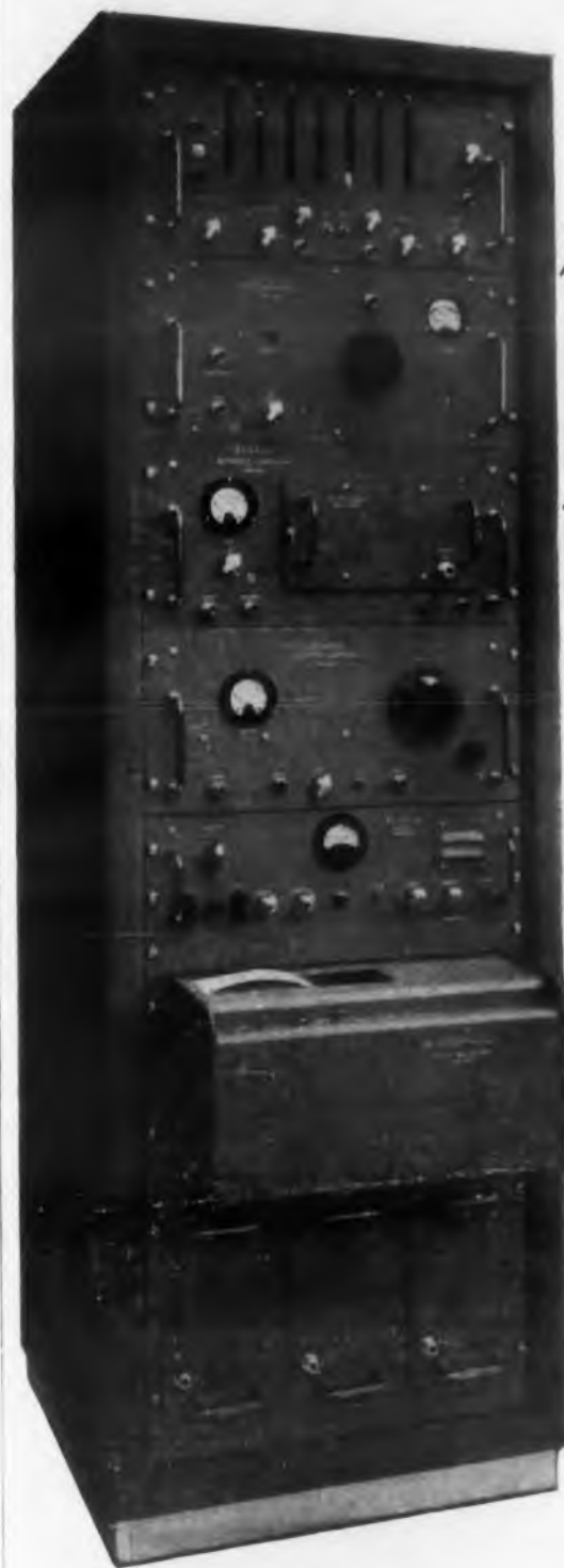
Typical automatic frequency measurement and logging system showing (top to bottom) Model 5571 Frequency Meter, Model 5580 Reference Generator with Model 5581 Plug-in, Model 5585 Selective Amplifier, Model 5590 WWV Receiver, and Model 1452 Digital Recorder.
