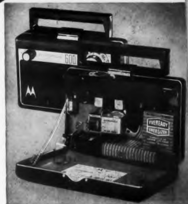
The Motorola "Ranger" achieves compact, sturdy construction and fast assembly with plated circuits on laminated stock produced by Farley & Loetscher Mfg. Co. , Dubuque, Iowa, using BAKELITE Laminating Varnishes.
