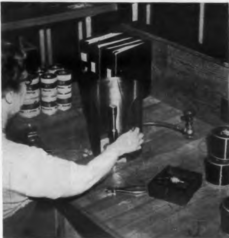
CLEANING THE INSULATION from enameled magnet wire, laboratory technician prepares to check conductor to see that it measures correctly after running through insulating machines.
