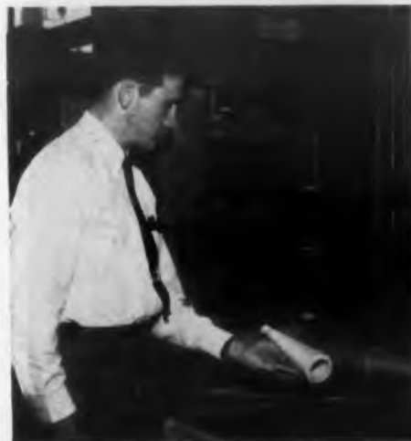
An engineer at Eitel-McCullough, Inc., holds sleeve of TEFLON molded by Chase Sales Company, Hayward, California, for use in klystron pictured above.
