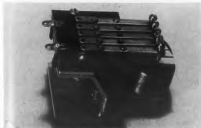
Resonant reed relay installed in a miniature radio control unit. Five auxiliary relays along the rear of the unit handle currents over the rating of the reed-relay contacts.
