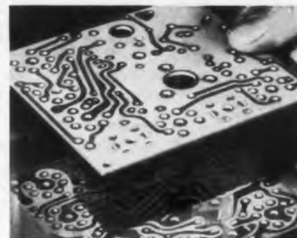
G-E "Thru-Con" Printed Circuit Boards offer positive connection through the holes, without staking pins. patterns on both sides if needed. Printed circuitry cuts assembly time; eliminates product bulk, weight; reduces inspection time, parts inventory.
