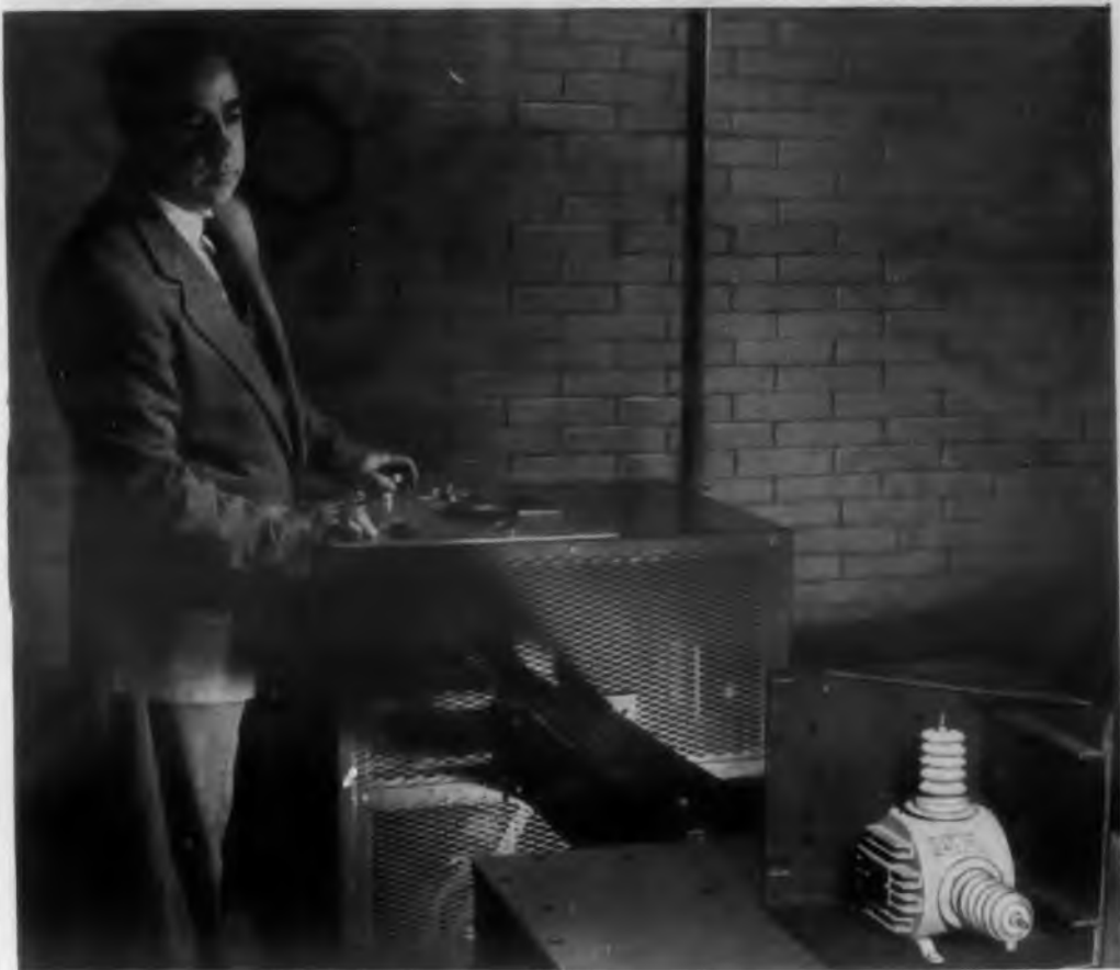
ONE OF MANY TESTS made on G-E oil-filled components is this six-hour vibration check.
