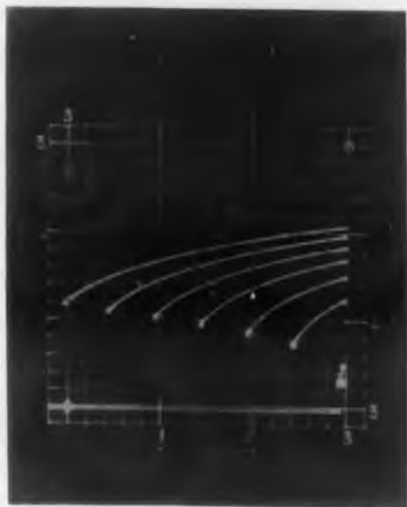
Fig. 6. Common-base emitter voltage vs collector current curves.
