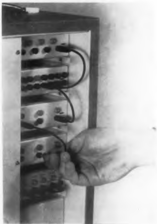
Patching or programming is made at rear of units.
