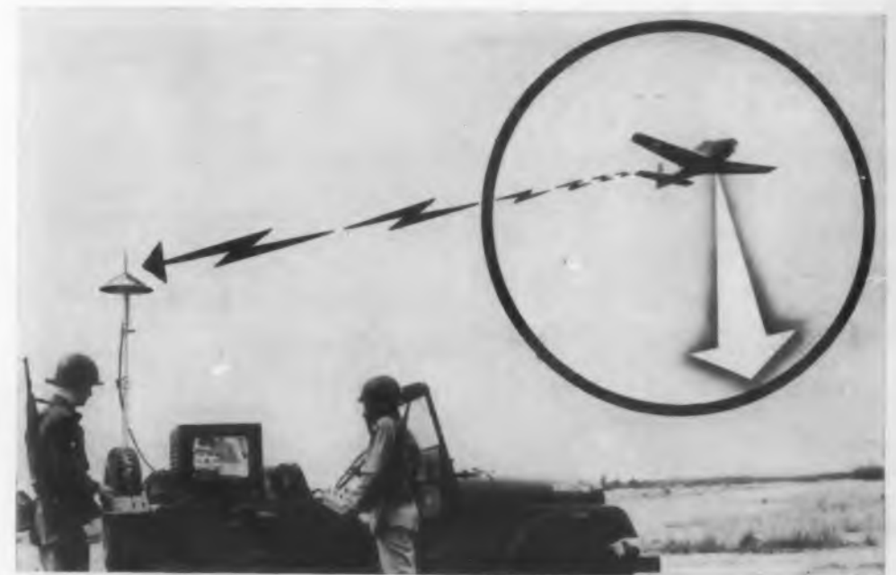
Soldiers operate radio remote controls that can pilot a TV robot plane up to 40 miles away. Soldier at left operates the plane's ground remote control box, while soldier at right works levers that point and focus aerial camera.
