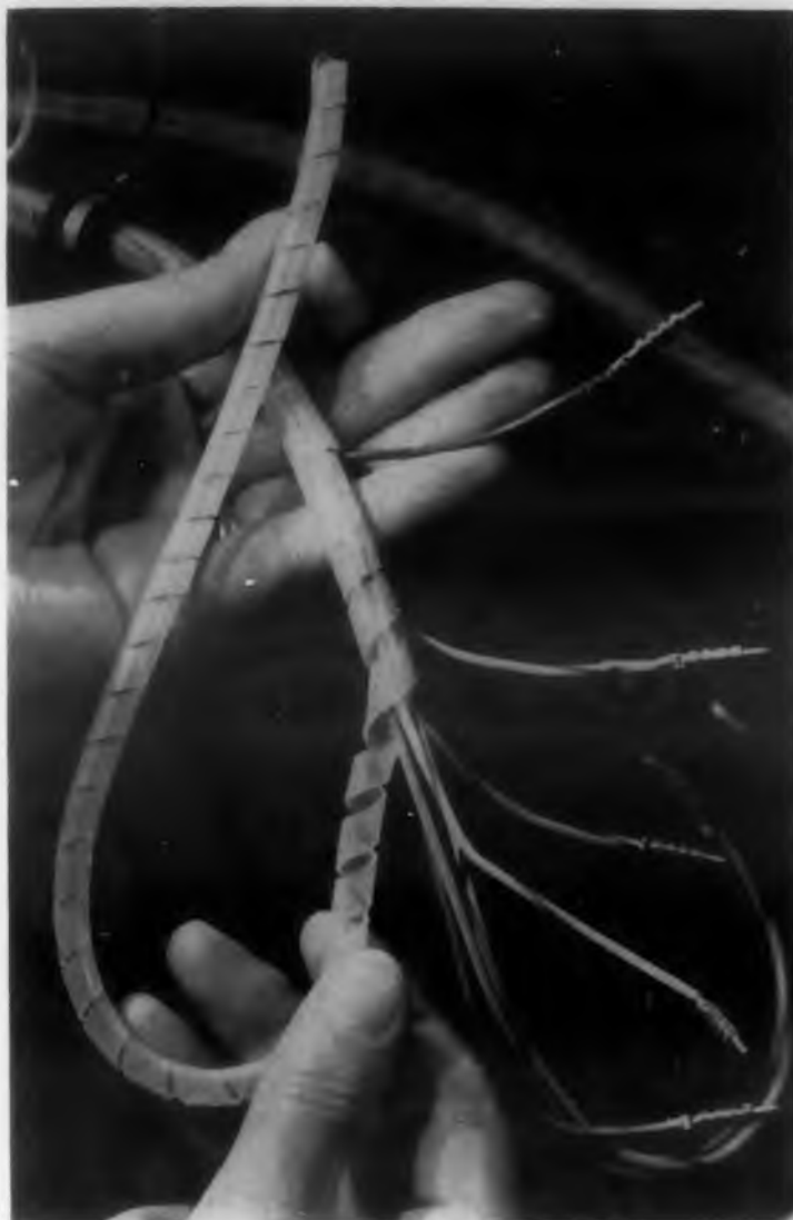
How spirally-cut plastic tubing is applied to a bundle of wires. Hand lacing with cabling twine is avoided.
