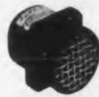
MODEL 162DA AXIAL FAN MOTOR —Totally enclosed, panel mount, screened intake, high temp. operation 20 CFM N.A.F.M. at free air. O.D. 1.45", 115 V., single phase, 400 cycle, or variable frequency models.
