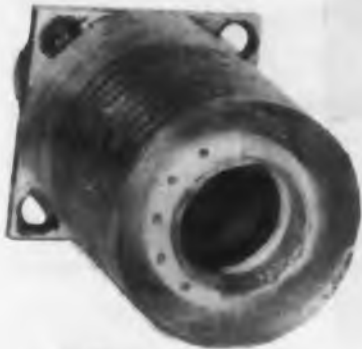
The groove has been covered with resin.
