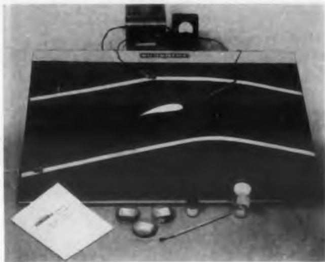
Analog Field Plotter set up to study flow around turbine blade.
