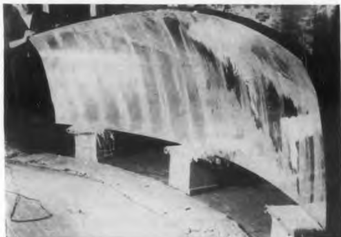
Aluminum reflecting surface of the fiber-glass reinforced antenna reflector for a taxi radar.
