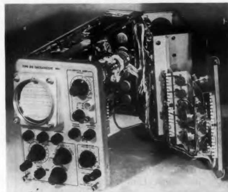
The 310 oscilloscope can be operated when hinged apart.
