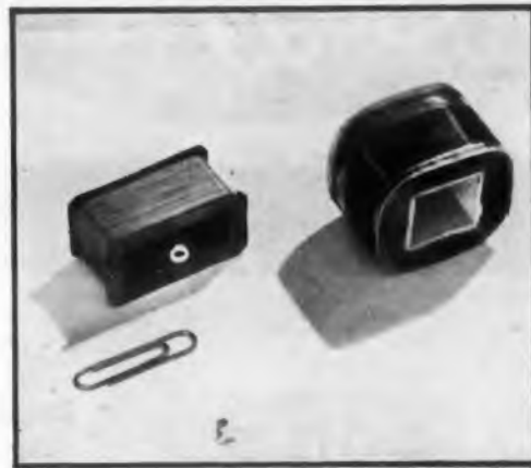
The paper clip indicates the small size of these coils. The insulation of "Teflon" is one important reason why they can be miniaturized.
