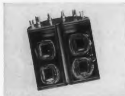
Section of magnetic amplifier coils embedded in Epon resin by Westinghouse Electric Corporation, Pittsburgh, Pennsylvania.
