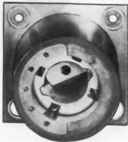
The tuning slug shorts out turns of the inductor.
