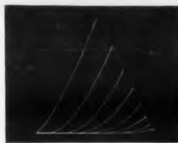
Fig. 1 — Plate current plotted against plate voltage for one triode section of a 12AU7. Plate load is 5 k, peak plate-supply voltage is 500 v. Grid voltage is changed 5 v between curves, from -35 v to zero. Vertical sensitivity is 5 ma/div, horizontal sensitivity 50 v/div. Calibrated controls permit accurate current and voltage readings directly from the screen.
