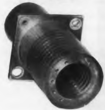
All the excess metal has been cut out of the interior to form the coil. The excess resin has also been removed.
