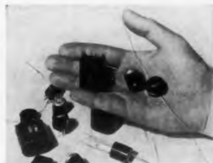
Miniature electronic components potted in Epon resin by Freed Transformer Company, Brooklyn, New York.
