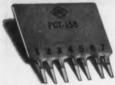
Centralab P.E.C. with 8 components
