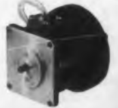
MODEL 430 AIRCRAFT DRIVE MOTOR —1/12 h.p. 11,000 r.p.m. Teflon insulation. -65° F. to +160° F. Completely qualified to MIL 7969 specs.
