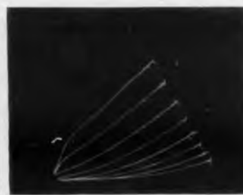
Fig. 2 — Same triode section of 12AU7 with only 20-v peak plate supply and sensitivities increased to 0.2 ma/div vertical and 2 v/div horizontal. Grid voltage is changed 2 v between curves, from -14 v to zero. This is essentially a 25-times magnification at the lower left portion of Fig. 1, showing the operating characteristics at low plate-supply voltage.
