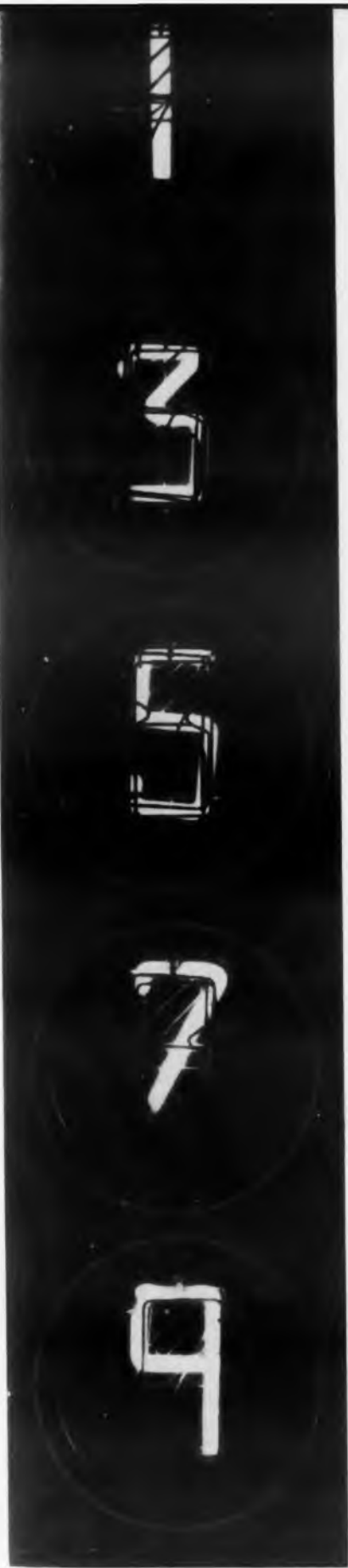
Fig. 2. (left). This is the way the numbers look when different elements of the indicator tube are energized.
