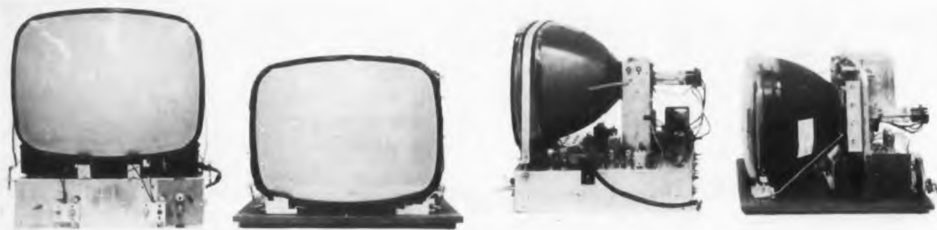
Fig. 2. The unique chassis construction and component arrangement of the unit compared with a standard receiver.
