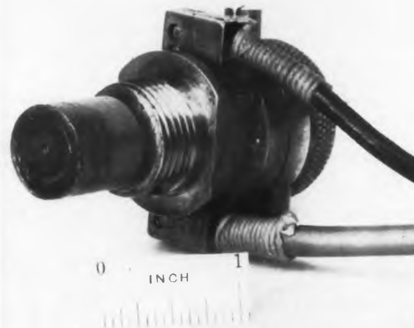
The mutual-inductance type micrometer used to detect thrust bearing wear.
