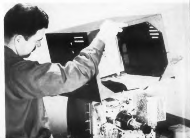
Fig. 3. To service the receiver, the cabinet is lifted off the chassis instead of pulling the chassis out of the cabinet.
