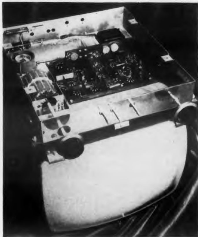
Fig. 1. The standard circuit of this 21" TV set was replaced by "Reliplates."
