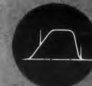
MARKA-SWEEP RF-P TV Tuner Alignment
