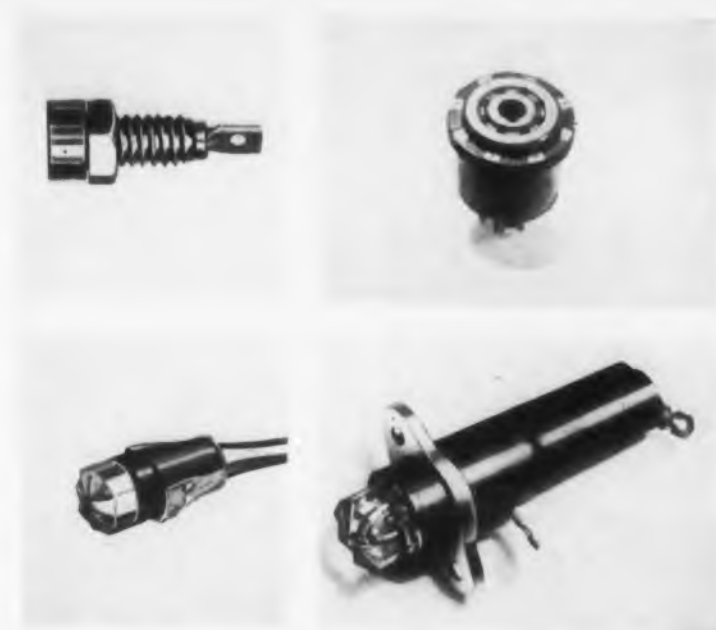
Fig. 5. Sensing elements: test point jack and plug-in adapter (upper left and right), panel light and indicating fuseholder (lower left and right) for locating trouble.
