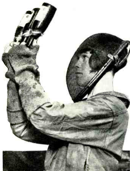
Girl workers in an English bottling factory are protected against exploding bottles by wire masks and thick woolen gloves.
