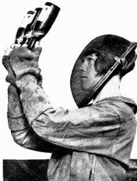
Girl workers in an English bottling factory are protected against exploding bottles by wire masks and thick woolen gloves.
