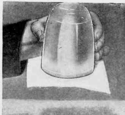
Left — The puzzling intermittent syphon can be simply made.
