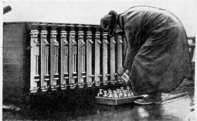
This battery of water bottles scoops up samples of sea water and automatically records temperature at different depths.
