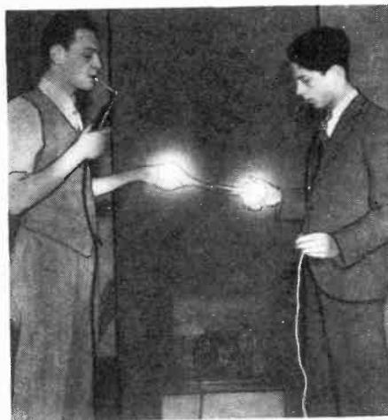
Fig. 5—The circuit is from the high voltage terminal to a nail in the subject's mouth. The high frequency current travels through his body and jumps to the lamp filament. Thence to the filament of the second lamp, to the hand of the individual holding it and to the ground through the wire.
