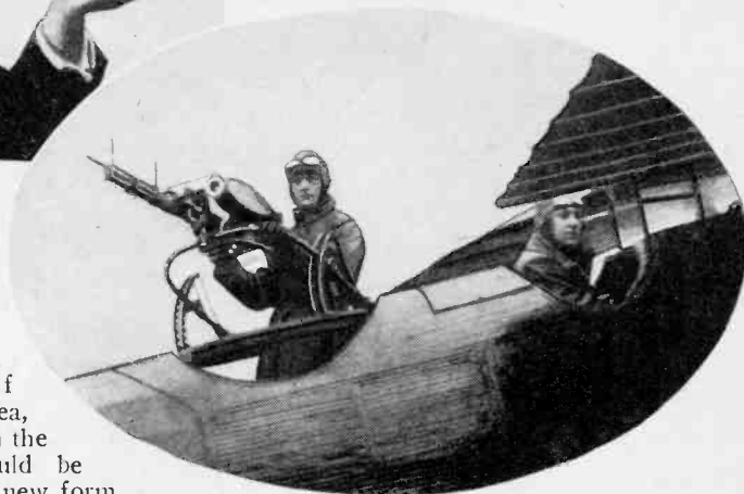
Above—The cinematographic "gun" invented by Professor Jules Marey in 1885. Right—A modern version of the movie "machine gun" as installed in the gunner's cockpit.
