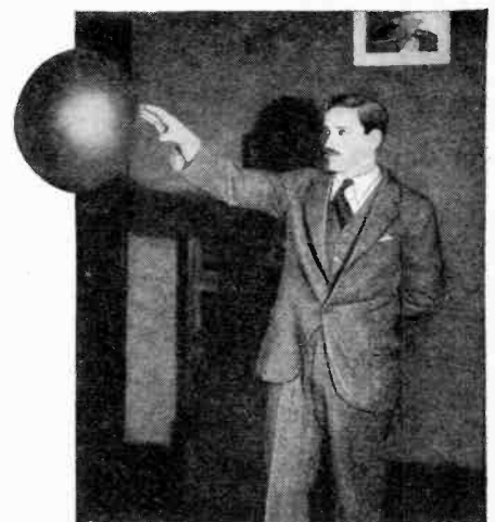
By properly charging a toy balloon electrostatically you can make it approach your extended arm.
