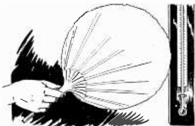
Fanning a thermometer to see whether there is any change in temperature.
