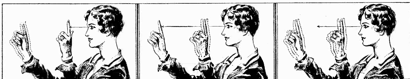
How three-dimensional effect is produced. Looking at near finger makes distant finger appear double and vice versa. Look midway between and both fingers appear double.
