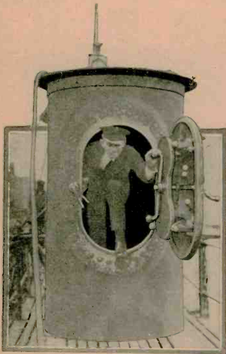
The above photograph shows a navy diver in the new escape lock device aboard the re-conditioned submarine S-4.
