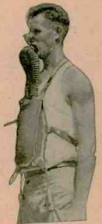
The above photograph shows a navy diver wearing one of the mechanical "lungs." Straps hold it in place.
