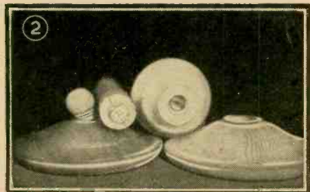
The turned base top and bottom portions for the lantern are shown above. The base and cap for the shade are turned in separate pieces and the work is done on the face plate.
