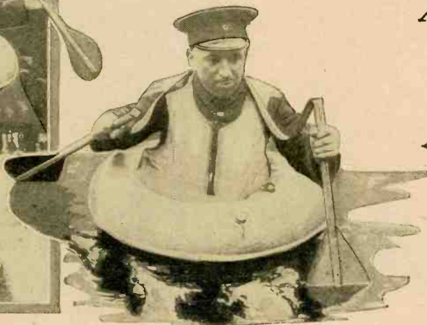
The photograph at the left shows a suit made entirely of rubber, which enables the wearer to walk in deep water. Successful tests were made by the Berlin Fire Brigade. Two paddles are provided.
