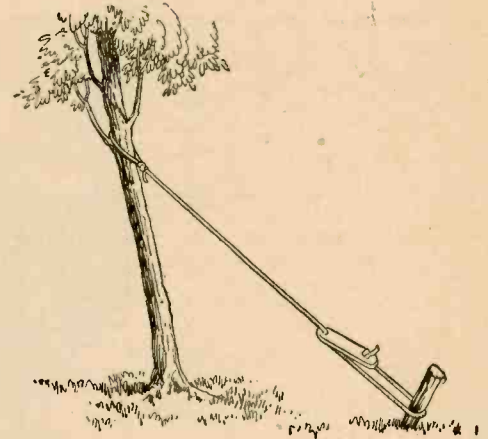
A leaning tree may be straightened to an upright position in a short time by using a tent guy-rope and a peg as illustrated. —Fred Cornelius.
