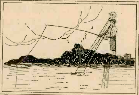
Diagram showing how optical refraction causes boy to appear taller than normal to fish under water.
