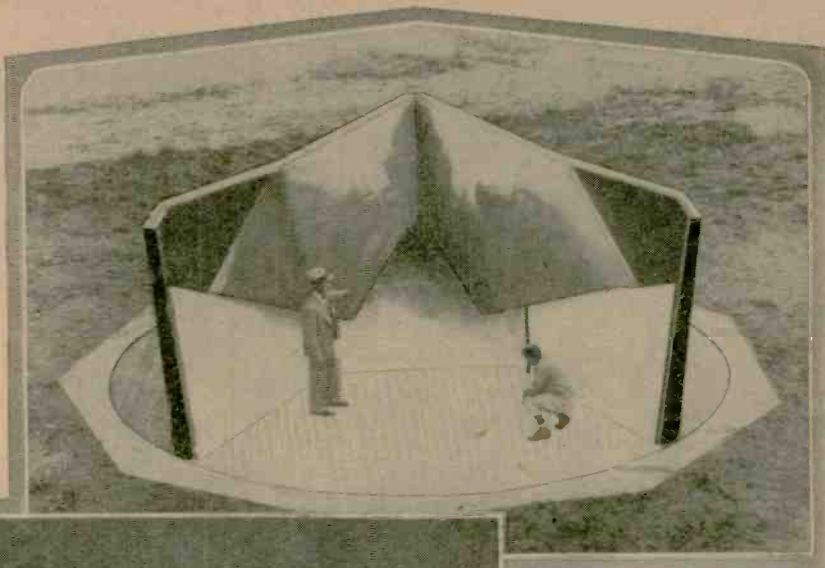
↑ Above — an invention for taking mail into speeding planes. A cable suspended from the plane travels along the ground into this device and catches a mail sack which is brought up to the plane by turning the cable drum.
