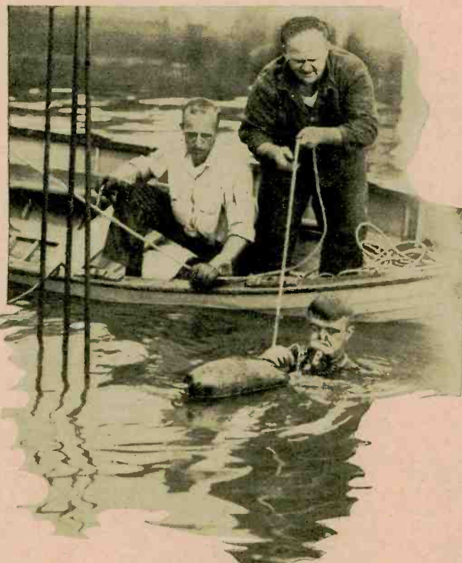
A diver is shown coming up to the surface during one of the tests made in the Potomac River. He has come up on the lifeline slowly so that he would suffer no injury from too rapid decompression. Note the lifeline buoy which the diver is grasping. The mouthpiece of the man-made breathing device can also be seen just above the surface of the water.
