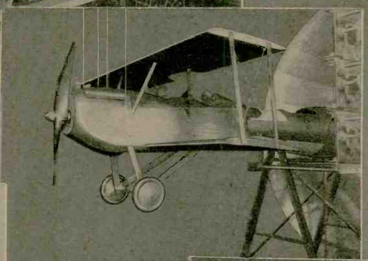
The photograph above shows a propeller ready for testing in a wind tunnel. A motor drives the propeller in a wind stream and by various instruments its effectiveness with and without an airplane model is determined. An airplane model used with testing propellers in wind tunnels is shown on the right. Note the supporting cables and portion of wind tunnel which appears at the extreme right hand side of the photo.
