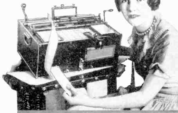
A device combining a talking machine and a visual chart which run in synchronism is shown above. Instructions are written as well as vocalized by the "portable tutor," an invention of A. L. Runyon.
