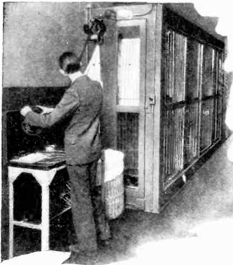
Roy Hunter, one of the inventors, watching the newly-invented film developing machine sending out the completed motion picture film, which is wound on reels by the machine.
