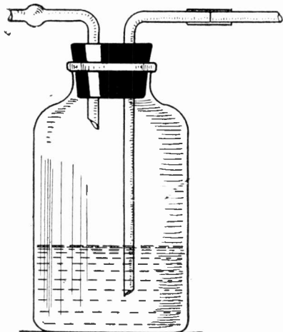
A variation on the chemist's wash bottle for the supply of distilled water, or of other liquids for laboratory use, a very convenient arrangement.
