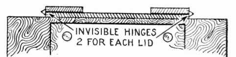
Constructional dimensions of the three drawers are shown above. Invisible hinges are used on each of the two top lids.
