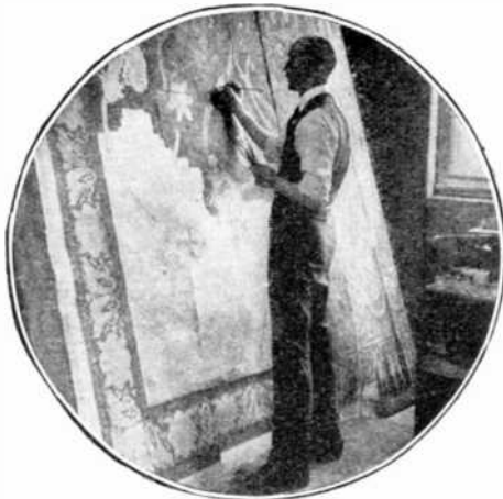
Fig. 1. "Starving" artist at work. Note 1,996,000 squares must be filled in by designer in 9' x 12' pattern. In a Karnak Wilton rug this takes from six to eight weeks.
