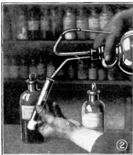
At the end of the minute add water to break the reaction and then thoroughly wash the nitrated cotton and dry in cool air.
