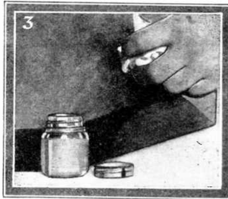
If vaseline is applied with considerable pressure to a finished surface, it will be found impossible to strike matches upon it. After applying, polish with dry flannel.
