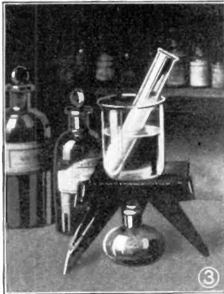
Mix equal parts of nitric and sulphuric acids, heat the mixture to 50° C (122° F) and add cotton. In ten minutes add water and wash.
