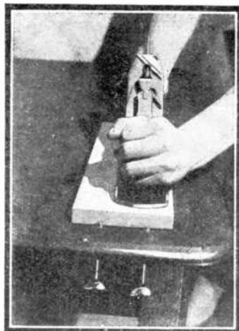
For planing upon the work table, use a simple bench stop as shown. It is constructed from two machine bolts with butterfly heads, screwed through the table top. They can be easily removed when not desired.
