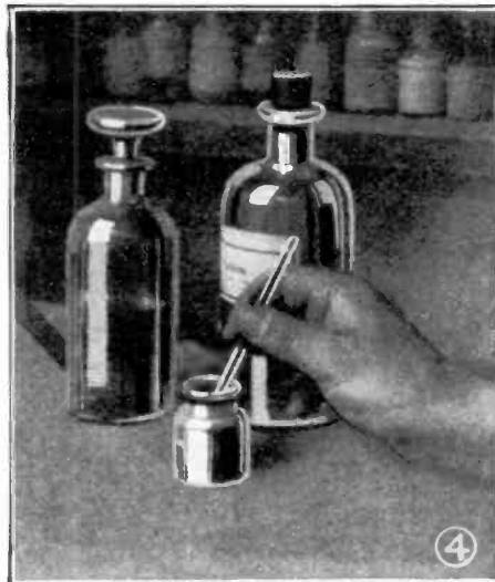
Make collodion by dissolving the lower nitrates in a mixture of alcohol and ether.
