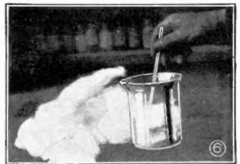
To the old solution add 100 grams of cotton by pressing the cotton firmly and strongly into the solution. Cover the flask or beaker and let stand for three days.
