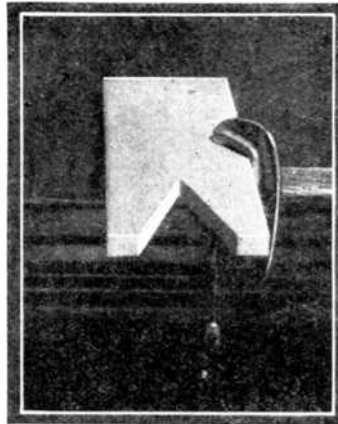
For filing, polishing, or trimming machined parts, a V-board makes an ideal rest. In the illustration above it is fastened to the table top with a C clamp.
