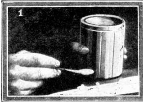
Dark wood which is to be bleached is first treated by the application of a solution of chloride of lime in water. A thick paste of this mixture is applied and allowed to dry.
