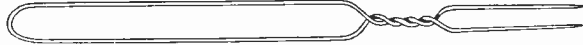
Thirteenth prize—$2.00. Here is a marshmallow toaster or bread toaster in the form of a fork. One single piece of wire, twisted as shown and pointed at the ends, finish the fork. This device was made by Burl Knutson of Bismark, N. D.
