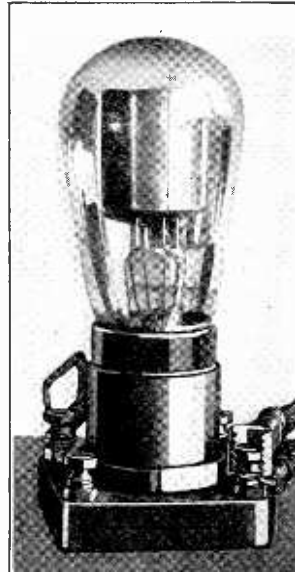
A photograph of the new "grid-glow relay," which is of about the same size as the ordinary radio vacuum tube.
