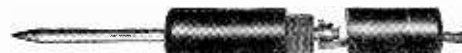
The thermoplex handle of the trouble shooter is shown above. The test handle is heat-proof, shock proof, moisture proof and will not warp.
