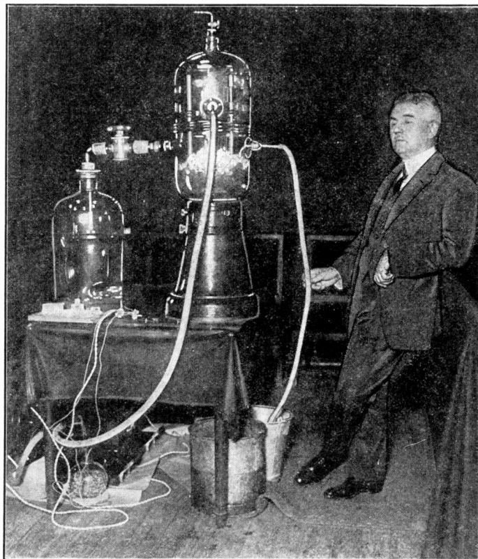
The above photograph shows Prof. Georges Claude who has developed a process for obtaining power from sea water. The apparatus in the picture is used for experimental demonstration of the principle of operation of this invention.
