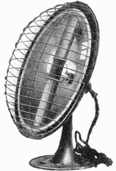
This heater combines the three principles in heat generation, radiation, convection and conduction. A tube passes through the heater and the heating coil is mounted in position at the center of the tube. Air is heated by the coil and circulates from the bottom through the tube and out at the top. A large polished reflector helps in radiation.—Dr. E. A. Martin.
