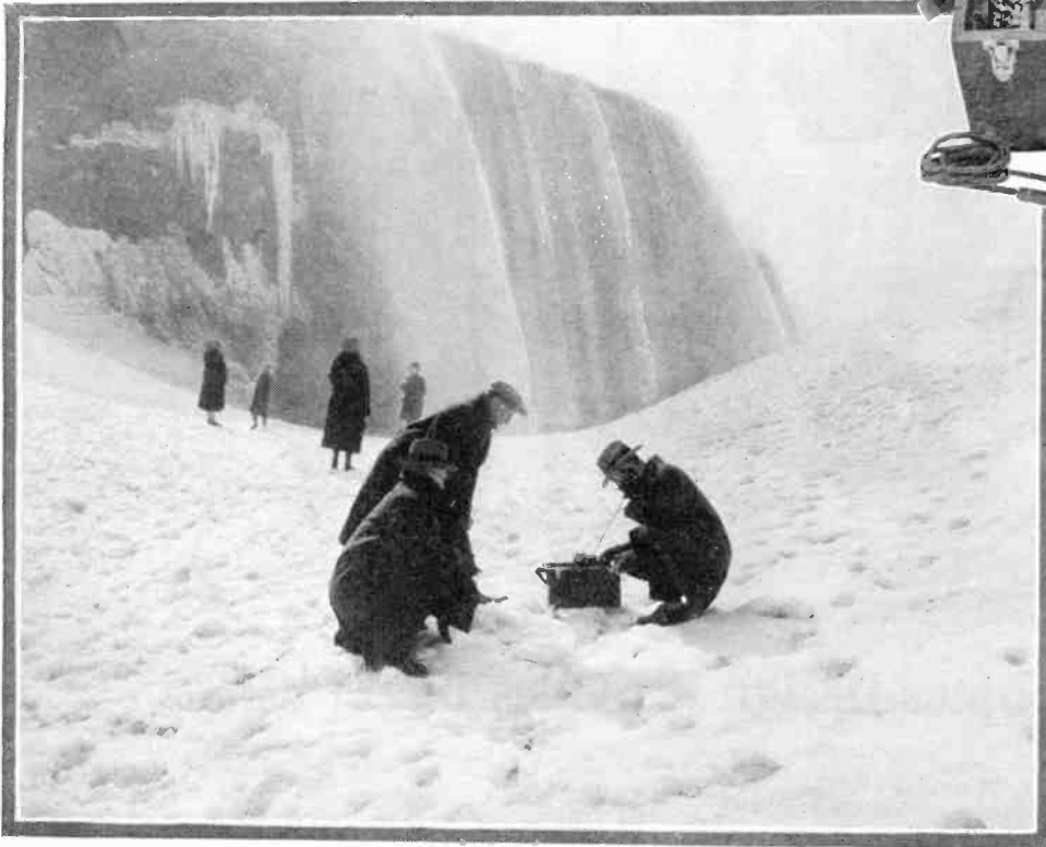
The interesting new instrument may be used with slight changes for the comparison of sound-intensities. In the photograph above two engineers of the Western Electric Co. are seen measuring the volume of sound at America's noisiest spot, the foot of the American Falls at Niagara.
