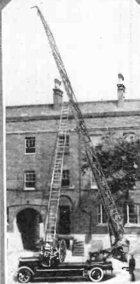
THE picture at the immediate left shows a remarkable new English turntable extension ladder, from which water can be played from a hose on to a fire. Note the nozzle at the top of the lofty extension ladder, which extends eighty-four feet above the ground. The photo does not do the apparatus justice, as this is one of the most beautiful pieces of fire-fighting equipment we have ever seen. It took some clever engineering design to get this whole affair balanced out, so that the ladder, when unfolded and extended upward, would not over-balance the truck which is extra-long as will be seen. The ladder resting against the building and provided with a two wheel truck, has no connection with the turntable extension ladder.
