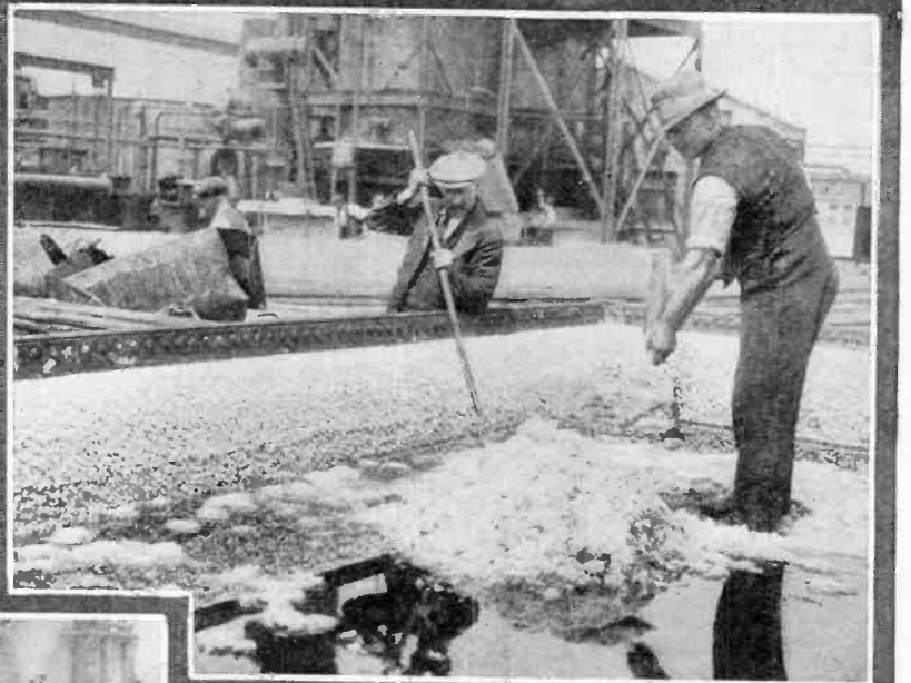
This photograph shows still another form of the use of old iron pots and pans. Here the employees at the gas works are scraping sulphate of iron crystals formed in the bottom and along the sides of a great tank. Some idea of the size of this tank can be gained from the photograph.
