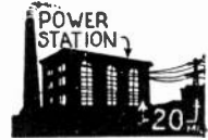
LOW VOLTAGE 500 TO 2000 VTS. D.C. OR A.C. TRANSMISSION, GOOD FOR 10 TO 20 MILES. WIRE 1/4" DIAMETER
