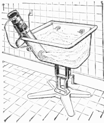
Here is a portable clothes washer weighing but 21 pounds which fits into any style of wash tub and will wash a tub-full of clothes in from 3 to 15 minutes. The clothes are washed by water alone, a powerful jet of water is driven through the fabrics which swirl about in the tub. The circular group of holes in the illustration are the intake and water issued from an opening at the center.—Freed-Eisemann.
