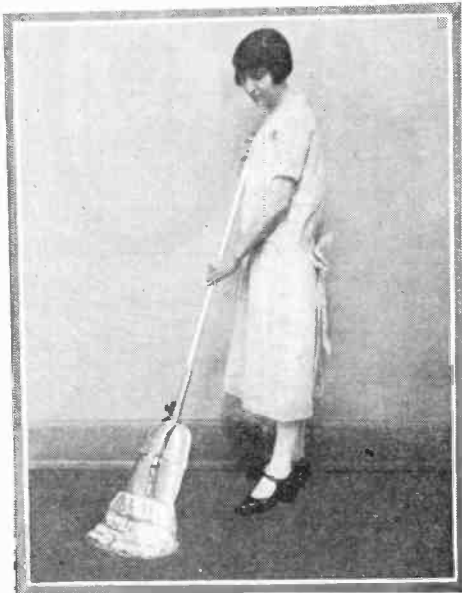
This is a simple invention which transforms an ordinary broom into a mop. The mop slips over the broom.—J. B. Roswick.
