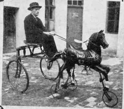
An exhibition of the latest German inventions, held recently at the Merkurhaus, Berlin, presented many new toys. One of the most ingenious was the trotting horse illustrated at the left, which is actuated by a mechanism concealed in the body. The motion is caused by pulling upon the reins while seated in the sulky. The machine goes about 3 miles an hour.
