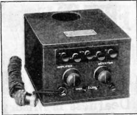
Appearance of latest style "B" Eliminator as furnished complete; ready to plug in light socket, by the manufacturers of the parts here described.
