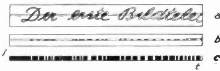
An illustration of how a simple design is transmitted. (a) One of the "picture lines" of the design to be transmitted. (b) The black and white dots of the "picture lines." (c) Represents the transmitted current of the "picture line."
