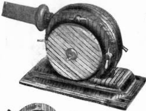
Fourth prize—$35.00 was awarded to the builder of this air turbine, Francis L. Lorenze, of Sayre, Penna. By blowing into the tube, this air turbine can be rotated at a humming speed. It may be instantly taken apart and reassembled as the next photograph shows.
