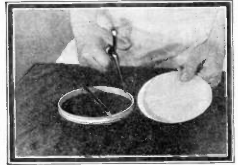
Fig. 3. The circle marked out in Fig. 2 should be cut out neatly with a pair of shears. A sharp razor blade makes a good tool to even up the edges of the disc so that it will fit closely into the hoop.
