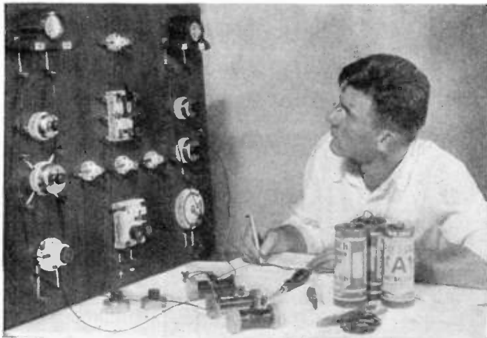
Measuring resistances by the use of a voltmeter and ammeter.
