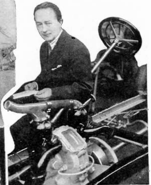
The sensation of the 20th annual automobile show in Paris was this tiny five horse-power, two-cylinder, two-cycle motor with no clutch or gears. To put the automobile in motion, it is only necessary to start the motor and press the accelerator, the connection between the motor and the wheels being made gradually through a system of governors actuated by centrifugal force. M. Constantinesco, the inventor, is also the perfecter of the method, much used in the world war, of synchronizing a machine gun to fire through an airplane propeller.
