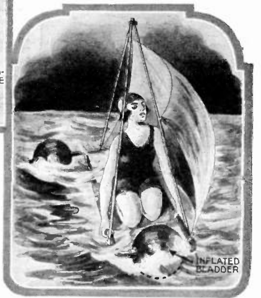
Devotees of water sports at British beaches this summer enjoyed the use of a cleverly devised aquaplane which is illustrated above. A frame, made of aluminum tubing, is supported upon the surface of the water by means of three large inflated bladders. The frame is extended upward to permit a sail to be stretched upon it and to afford a hand-hold.
