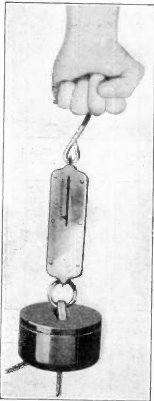
By means of a spring balance the pull of the electro-magnet provided with the study course, is obtained.
