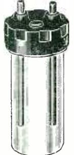
These rectifier cells, of which four must be used for the complete full-wave rectification, are standard with us, having been specially designed for "B" eliminator work. These 4-oz. jars, with acid- and heat-proof rubber screw covers, are furnished with two electrodes, namely pure aluminum and lead. A vent cap is also provided. The special connectors listed below should be used for connecting the cells together. Size 4 1/2" x 2 1/4".
