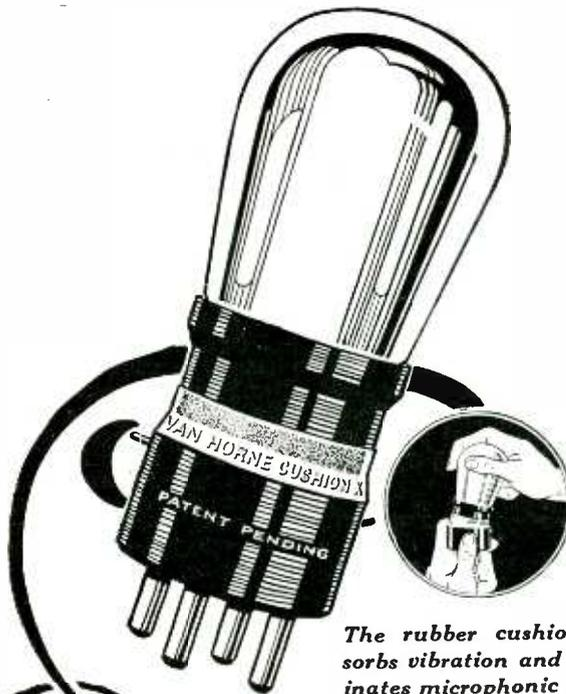
The rubber cushion absorbs vibration and eliminates microphonic noises
