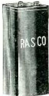
These are standard condensers and are of the best vacuum impregnated paraffin type. The insulation is specially-prepared paper, and the units are compressed hydraulically before they are sealed in their metal casings.
