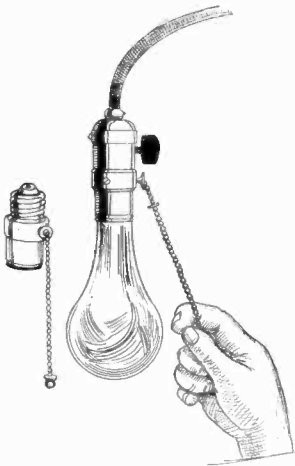
Any kind of a socket can be converted into a pull chain socket by screwing the adapter here shown into it. The advantages of the pull chain can thus be obtained without the need of re-wiring the fixture. Courtesy Bryant
