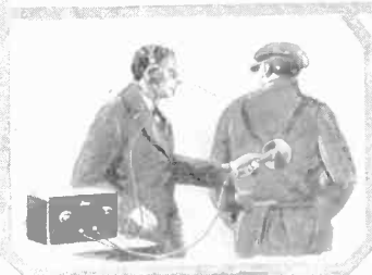
An apparatus for searching the employees of metal working establishments when they are leaving the premises has recently been devised. This consists of a testing disc containing a pair of coils. A distinct sound is heard in the headphones when the disc passes over metal. The method is undoubtedly similar to a Hughes Balance.
