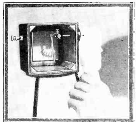
Friction produces electricity, as can be seen by the divergence of the gold leaf when the connecting post is smartly whipped with a dry handkerchief.
