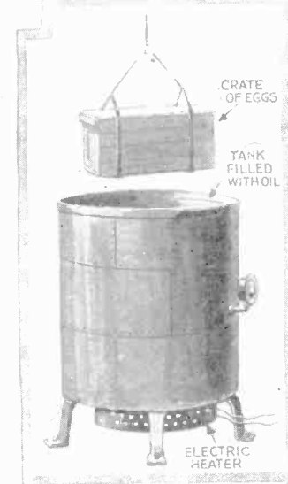
The laboratory of the General Electric Company at Schenectady has just announced a method of egg preservation which consists of immersing eggs in an oil bath maintained at a temperature of 235 deg. Fahrenheit. The oil is said to fill the pores in the egg shells and prevent air from entering the shells. The machine is electrically equipped and accommodates 360,000 eggs per day.
