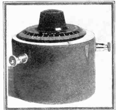
A panel type condenser may be adapted for table mounting by fastening it inside of a piece of cardboard tubing by means of a pair of brass brackets. Connections are made to binding posts and a cardboard top is put on the tube.
