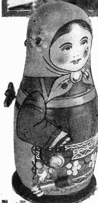
A Russian concern has recently produced a crystal set built inside of a hollow manikin. The controls are almost inconspicuous, blending with the designs on the figure.
