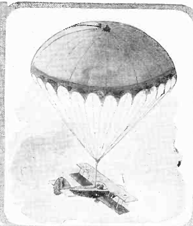
While a number of inventors have advocated the use of a large parachute for the purpose of saving a falling airplane, here is the latest idea for such a device.
