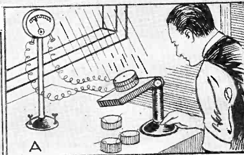
The sunlight shines through a pin-hole in the top of pill box on to sensitive spot on surface of molybdenite strip. As long as the sun shines on the molybdenite, a deflection is noted in the galvanometer. Connecting several of the strips in series yields an increased voltage.
