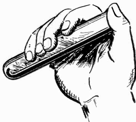
Agitating the solution. This is an efficient way of doing it, but see that your thumb covers the mouth of the test tube or the contents will fly out.
