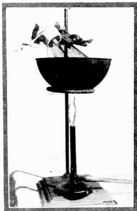
Arrangement of the iron dish containing sodium nitrate melted by a Bunsen burner and the incandescent lamp bulb partially immersed in the melted salt and supported by the same retort stand as shown.
