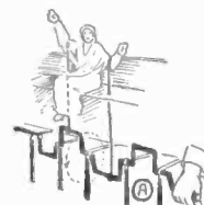
TURNING CRANK "A" CAUSES ARMS OF DOLL TO RAISE AND LOWER ALTERNATELY
