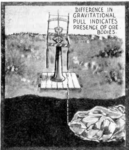
Fig. 3. The above illustration shows the method of using the Eotvos Torsion Balance. This was designed by Baron Roland von Eotvos of Budapest. It is placed near to the edge of a supposed mineral ore area, and due to difference in gravitational pull, indicates the presence of these bodies beneath the surface of the earth.
