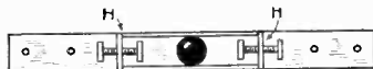
FIG. B - TOP VIEW OF ARMATURE This shows the top of the beam with the ball, this time, in the central position, and on the point of traveling toward one or the other end, actuated by the current received. This lever constitutes the armature.
