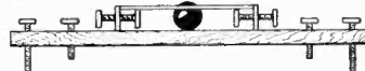
FIG. C SIDE VIEW OF ARMATURE This gives the side view of the oscillating armature, showing the ball in the central position, as above, on the point of rolling to right or left.
