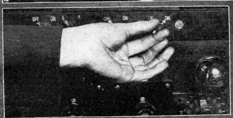
And in the broadcasting station, when orders are issued to stop for an SOS, a snap of the switch shown in the photograph above immediately takes the station off the air and clears the way for rescue messages.
