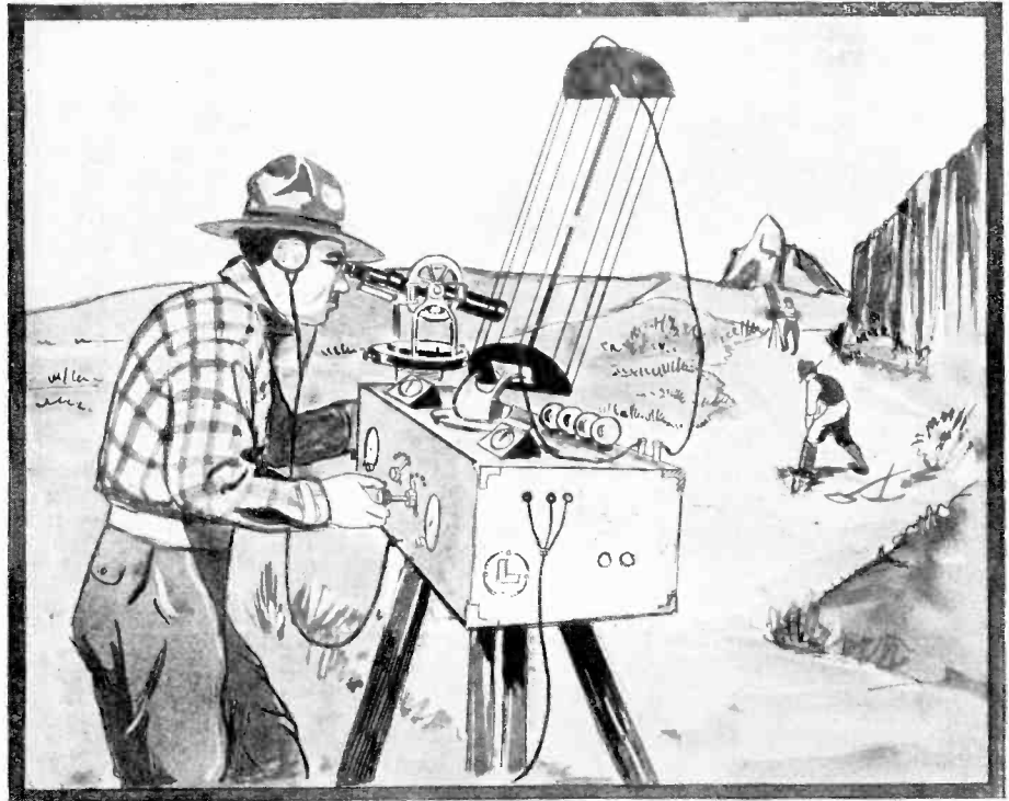
Fig. 4. The above illustration shows the radio gold explorer in operation. The directive radio beam being sent out from the apparatus in the distance, which at the present time is being used as the transmitting end, is picked up at the set in the foreground. The beam from the transmitter is reflected by subterranean ore bodies or chests of gold. By means of the surveying instruments the exact position of the hidden treasure can be pointed out and attempts to secure it can easily be made.
