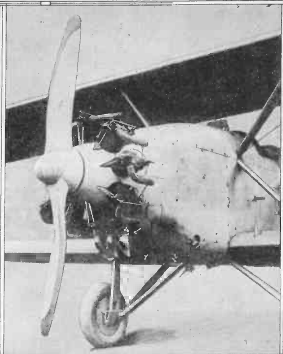
↓ A new type of radial cylinder air-cooled engine of low weight to horse-power ratio has recently been completed, having been designed especially for the United States Bureau of Aeronautics. One of the engines, delivering 450 horse-power, was substituted for a 400-horse-power Liberty engine with a saving in weight of 285 pounds and a great increase in performance.
