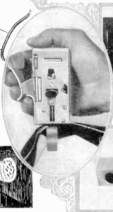
For stenographers who take a great deal of legal dictation or other such work, this knee shifter will be found exceptionally handy and a great ease to the hands. This attachment may be applied to any ordinary typewriter and greatly facilitates the stenographer's work. —Lester Sargent.
