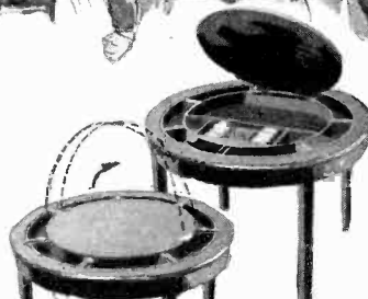
Many card clubs use tables fashioned after the plan of that shown above. It spins over, hiding the evidence of the game in case the police pay an uninvited call.
