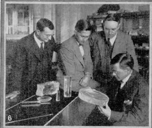
Above are shown some of the forms into which the fused quartz has been worked. The large circular piece, which the gentleman at the left of the photo is holding is worked into lenses, such as those shown at illustration 2 above. The quartz, having coefficient of expansion much lower than that of glass, will not break with the quick changes of temperature inflicted upon it by such uses as condenser lenses for motion picture machines, etc., are subjected to. The other subjects in the above illustration show how the quartz may be brought from the furnace. Afterward, it is worked into desired shapes in much the same manner as glass, with the aid of a gas flame and a blow-pipe.
