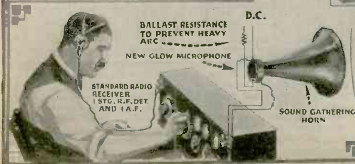
OUTLINE OF GLOW DISCHARGE MICROPHONE The curved unit shows what is termed an "exploring electrode"
