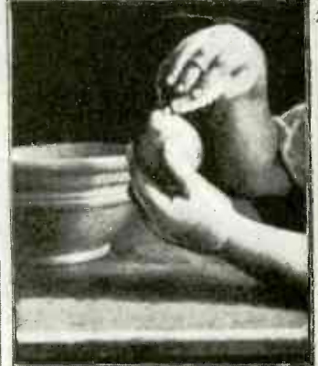
The handy potato peeler shown above is simply a rough carborundum stone compound placed in a tin receptacle on the back of which is small loop which fits over the finger.
