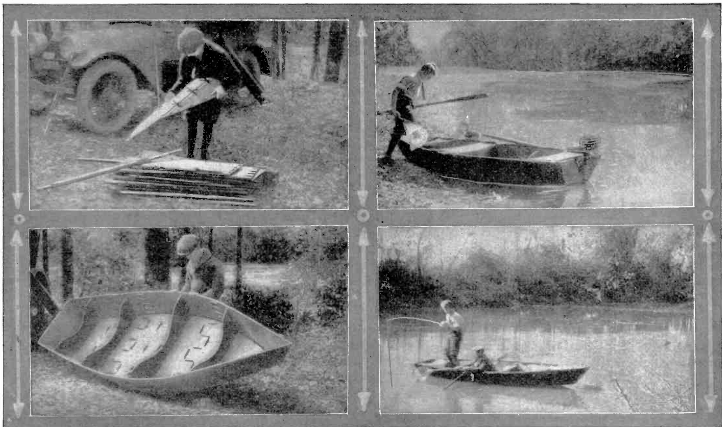
Weighing less than 100 pounds and packed in a case 12 by 18 inches when not in use the boat shown in the above photographs is capable of carrying three persons. It is built of laminated three-ply wood and is covered with heavy canvas to make it water-tight when
