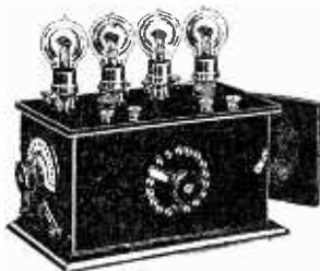
A French set of a compact type is shown above. The inductive relation between the primary and secondary coils is varied by moving the right hand end of the box, which is on hinges.
