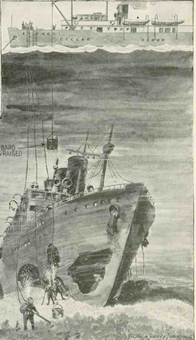
As Our Front Cover Illustration Shows, this New Invention for Locating Sunken Ships Can Be Operated Without the Aid of Divers or Diving Machines. It is Based on the Hughes Induction Balance, Where a Slight Change in the Induction Between Four Balanced Coils Causes a Sound to Be Heard in One of the Circuits.
