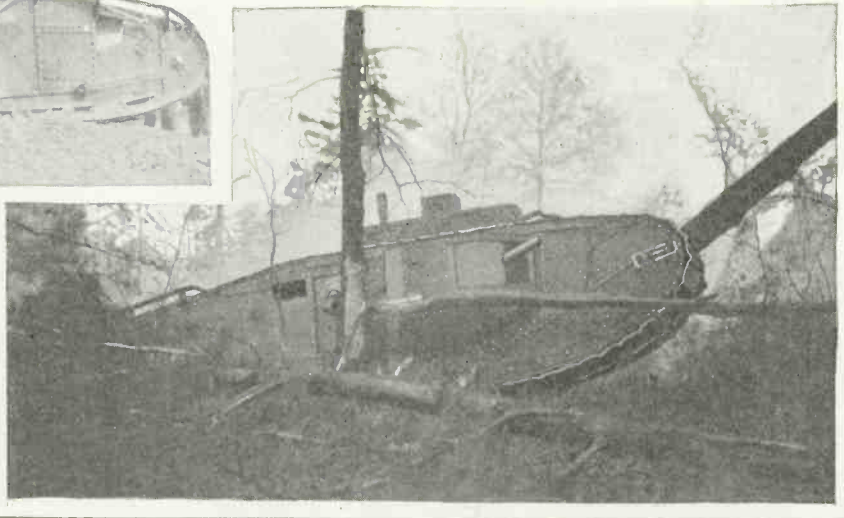
Ordinary Houses and Trees 12 Inches in Diameter Are Knocked Down by the New Mark VIII Tank. Its Path is Readily Followed by the Light Tanks and Infantry and Can Easily Be Made Usable by Supply Vehicles. The Engine is a 400 H.P., 12 Cylinder Liberty Type Geared Down. Lower Left Picture—Radio Controlled Tank—of To-Morrow.
