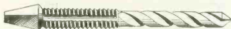
The combination drill and tap idea shown above is very old. It has been found inefficient.
