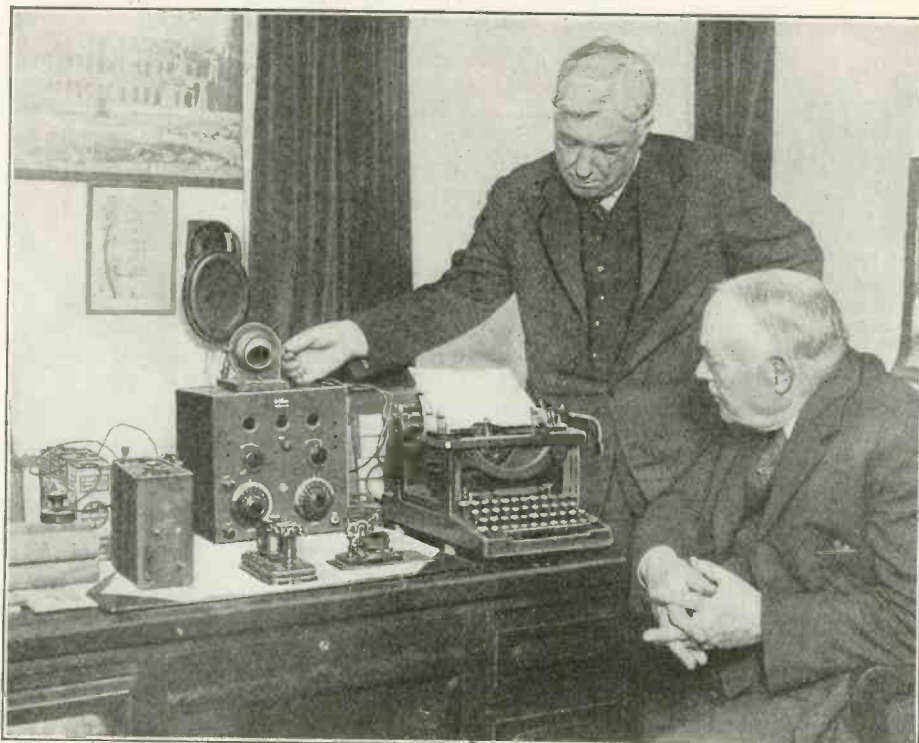
New Intercommunicating Electric Typewriter Invented By Dr. George A. Cardwell of Yonkers, New York. A Station With Such a Typewriter May Communicate By Wire With a Similar Station.
