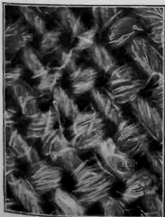
Notice the Fibers in This Linen Cloth Magnified 375 Diameters. The Wonderfully Even Illumination is Obtained by the Lighting Device at the Right.
