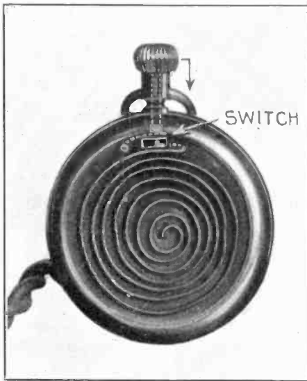
Electric Cigar Lighter Built into a Watch Case. It Works from the Car Battery.
