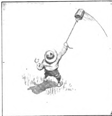
Fig. 3—Swinging a Pail Containing Water in a Circle Will Cause the Water to Remain in the Pail Due to the Centripetal Acceleration. With a Cord Three Feet Long the Pail Must Revolve Twice per Second in Order to Retain the Water.
